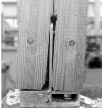
Figure 2.7. Post base joint with concealed connector (Humbert et al., 2014)
