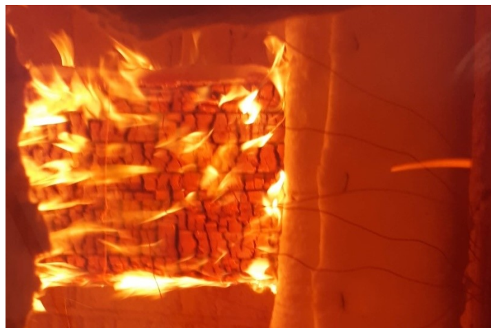
Figure 5.5. Beam-to-column connection assembly exposed to 30 minutes of a standard fire
