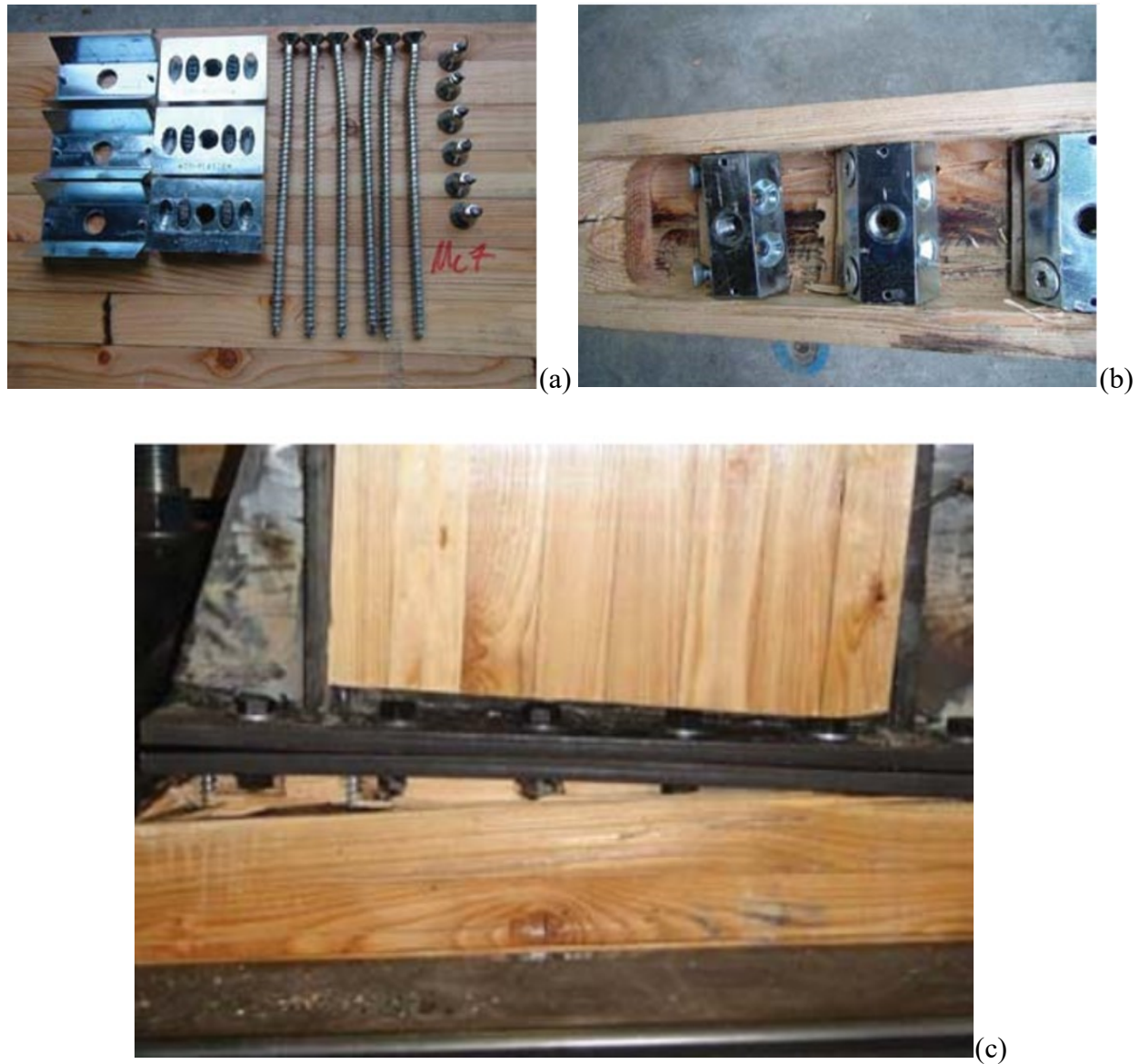
Figure 2.5. Failure modes of self-tapping screw fastening beam-to-column connection: (a) disassembled ZD-plate with compression screws bending and tension screws fractured removed from beam section; (b) disassembled ZD-plate with compression screws bending and tension screws fractured attached to beam section; (c) Screw withdrawal in bottom member (Closen and Lam, 2012).
