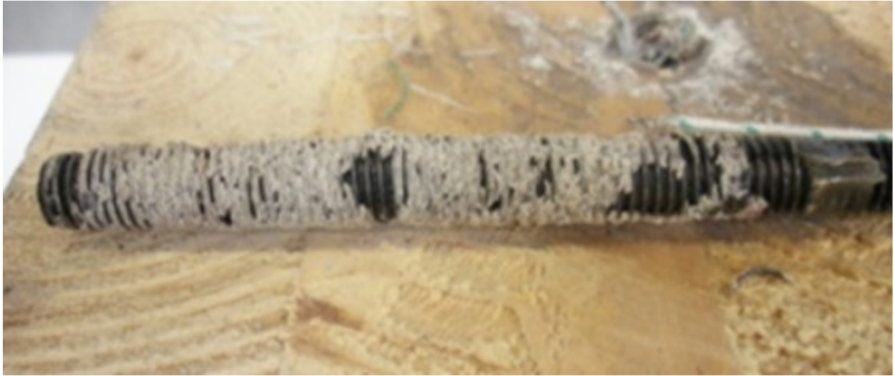
Figure 2.15. Crumbling effect of epoxy resin after being exposed to elevated temperatures (Di Maria et al., 2017)
