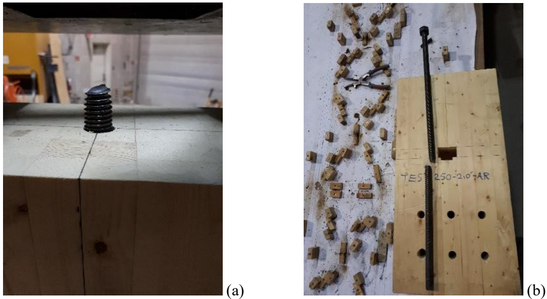
Figure 3.22. Yielded steel rod and non-deformed glulam section: (a) Steel rod broken in glulam; (b) Fractured steel rod.
