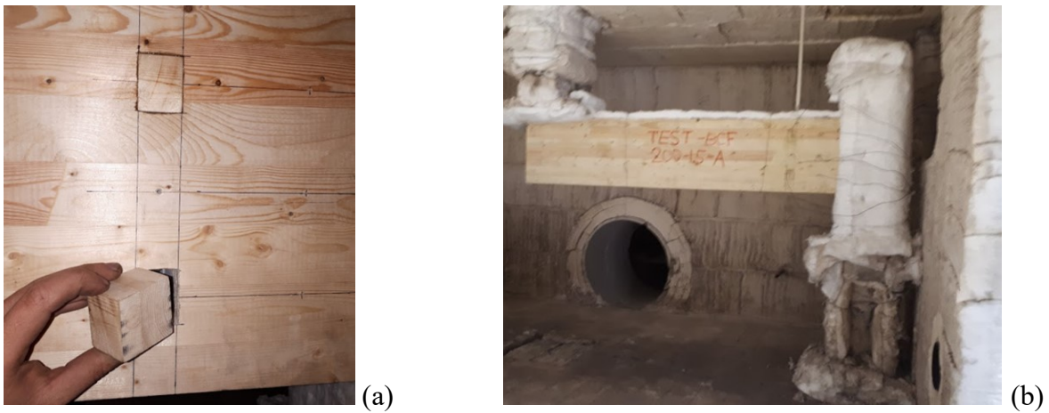
Figure 5.2. Fire test setup: (a) Beam section holes being plugged; (b) A general fire resistance test setup.
