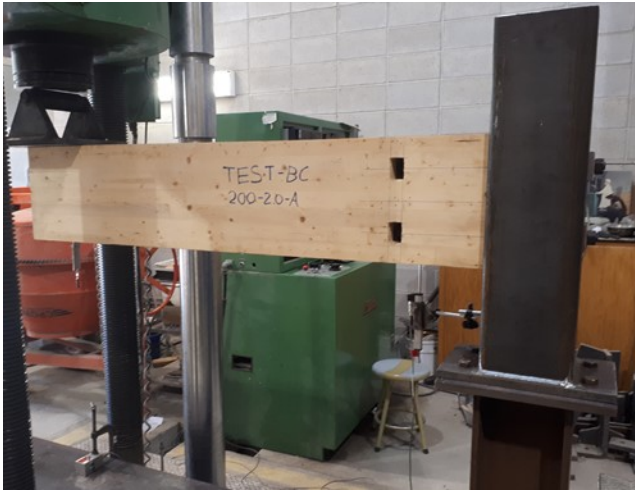
Figure 4.4. Full test setup of a general beam-column connection test assembly: (a) Full test assembly diagram; (b) Front side of assembly setup; (c) Back side of assembly setup.
