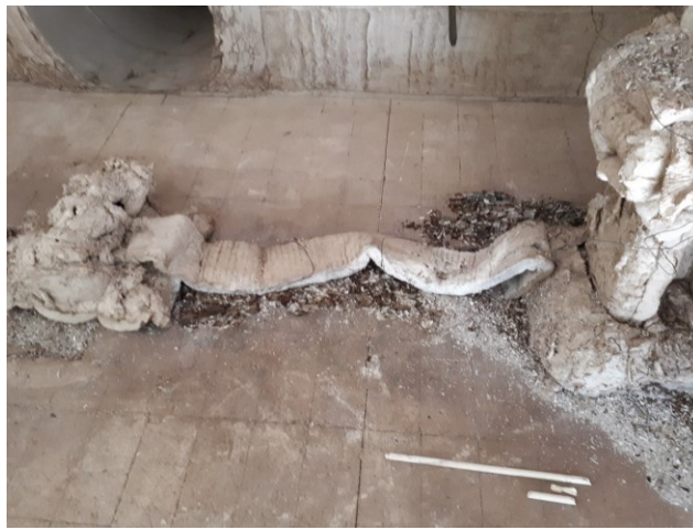
Figure 5.6. Fire tested beam upon completion of testing
