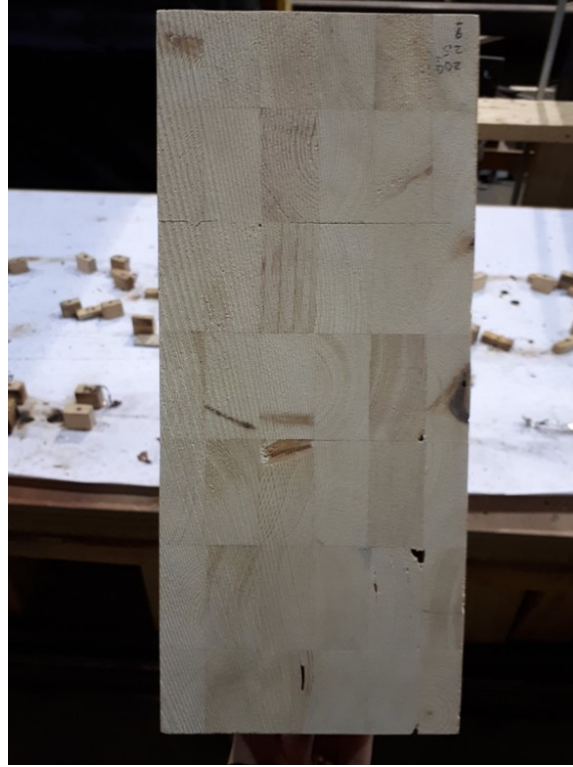
Figure 3.1. 135 mm x 314 mm glulam beam cross-section
