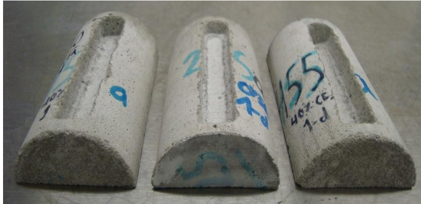
Figure 2-1 Split mortar cylinders showing grooves from material removed by the drill press for the FTIR and dust digestion methods.
