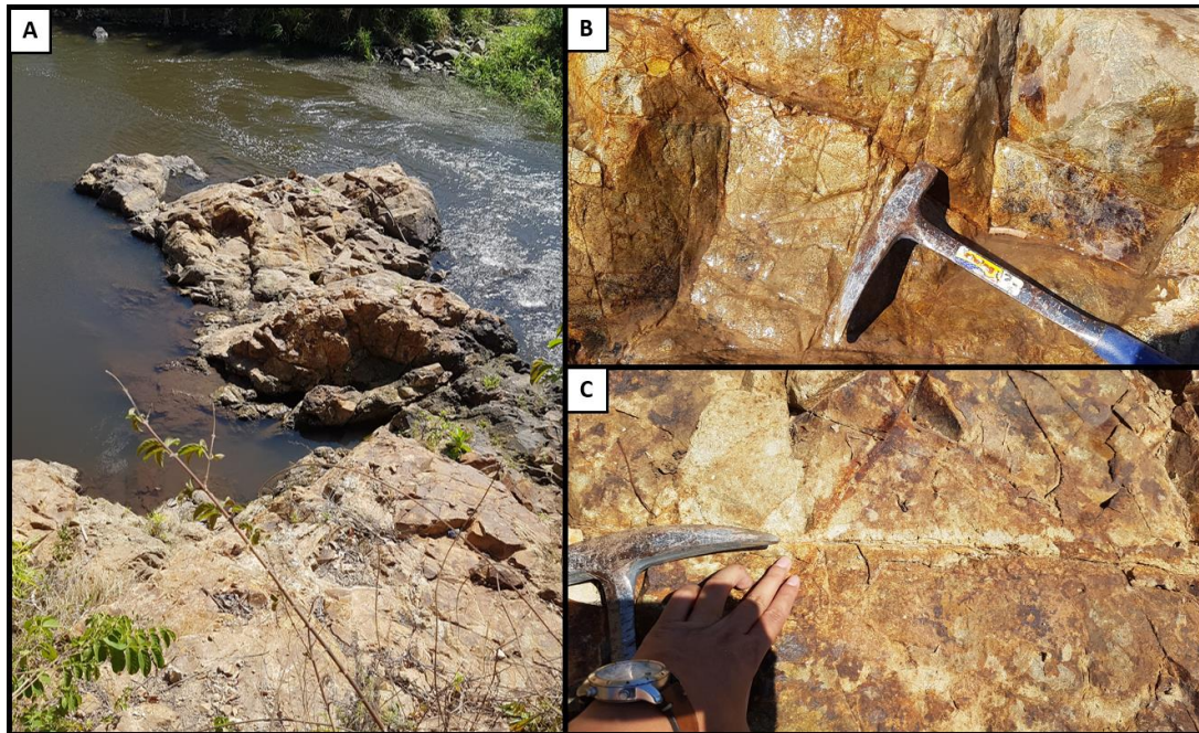
Figure 4.21: (a) outcrop of quartz diorite porphyry in the Mandilis River (JEM-02). (b) Quartz stockwork in JEM-02. (c) Goethite and jarosite veinlets. Photos courtesy of Adi Maryono.
