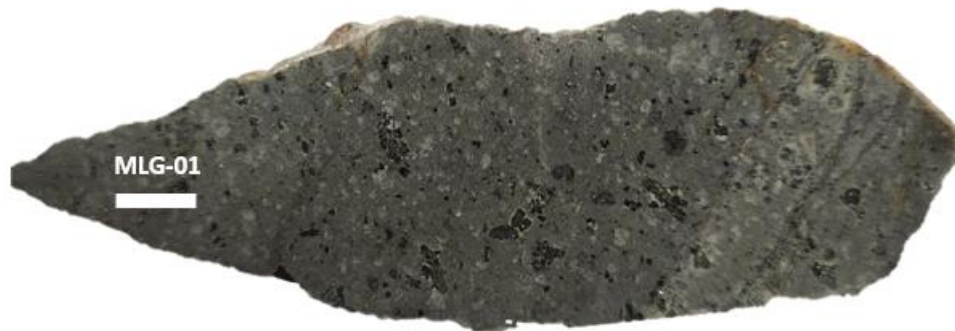
Figure 4.19: Photograph of andesite porphyry (MLG-01) from Malang, Java. White scale bar is 1 cm.
