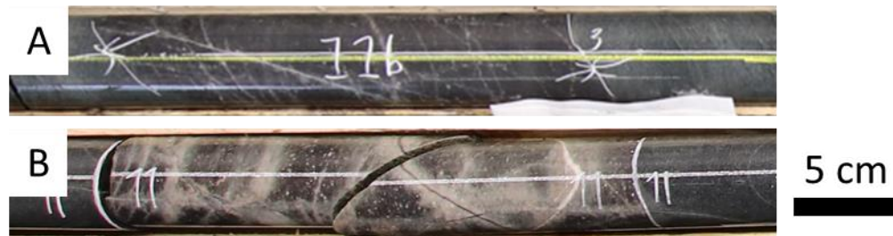
Figure 5.28: Chaotic unit hosted within feldspar porphyry unit (ERX-2021-56 @ 251m; a); and alteration variability as it progresses from the feldspar porphyry unit into the volcanic rock (ERX-2021-71 @ 139m; b).
