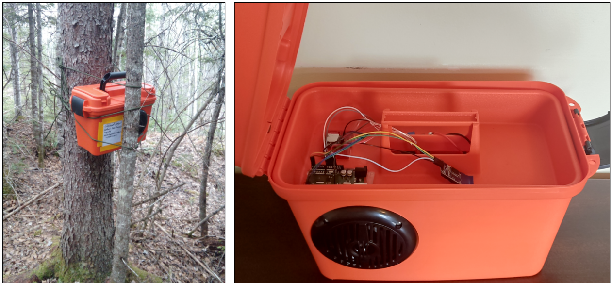
Figure 4.2. Automated speaker system (Cupiche et al., 2023) installed for a minimum of seven days on each site. Left picture: speakers installed in the field. Right image: an overview of the speaker system used (microcontrollers, speakers, and battery inside a waterproof box).
