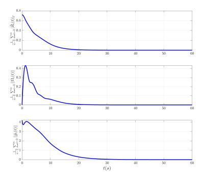
Figure 3.7: Time evolution of the average estimation error norms considering the observer (3.8)-(3.9), (3.14).
