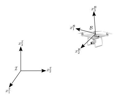
Figure 2.3: Coordinate systems:  $\mathcal{I}$  is the inertial frame and  $\mathcal{B}$  is the body-fixed frame attached to the center of mass of the VTOL aircraft.
