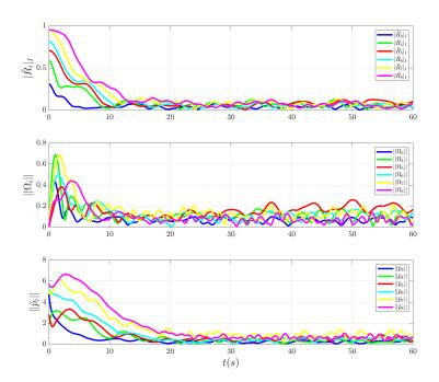
Figure 3.10: Time evolution of the individual estimation error norms for the observer (3.8)-(3.9), (3.14).
