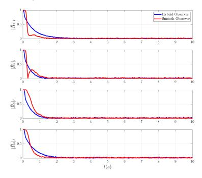
Figure 4.6: Time evolution of the relative attitude error norm, associated with each edge, for the *Continuous observer* and the *Hybrid observer* using noisy measurements.
