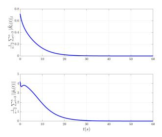
Figure 3.5: Time evolution of the average estimation error norms for the observer (3.3), (3.14).
