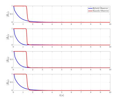
Figure 4.4: Time evolution of the relative attitude error norm, associated with each edge, for the *Continuous observer* and the *Hybrid observer*.
