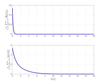
Figure 3.15: Time evolution of the average estimation error norms.
