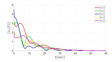
Figure 4.9: Time evolution of the relative position estimation error norm.
