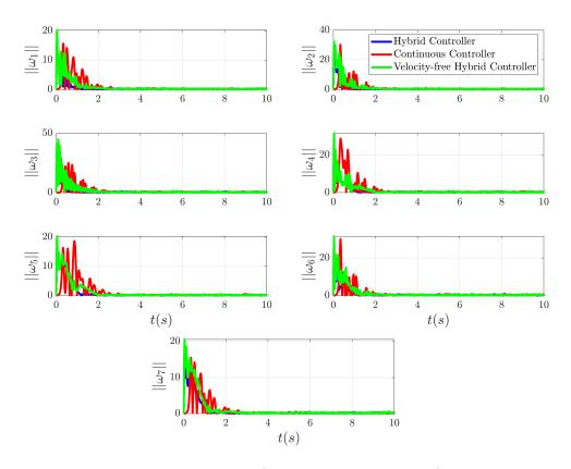
Figure 5.9: Time evolution of the angular velocity of each agent.
