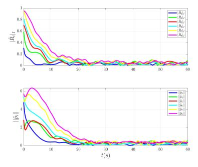
Figure 3.8: Time evolution of the individual estimation error norms, with noisy and biased measurements, for observer (3.3), (3.14).
