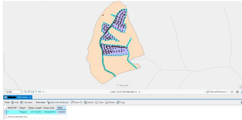
Figure 7. Shows the outline for Block 2 along with the calculated polygon area (ha) around the tracks of FB23.
