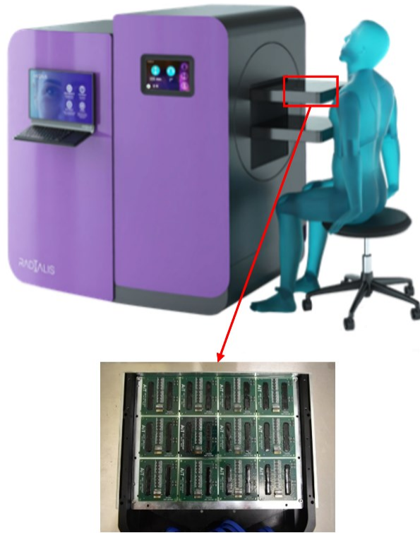
Figure 17. Top: Radialis PEM camera with two planar detector heads positioned horizontally on both sides of the immobilized breast for imaging in the craniocaudal (CC) view. The detector heads can be lifted, with the separation between them adjusted to allow rotation and acquisition of images in the mediolateral oblique (MLO) view. Bottom: 3 \times 4 array of sensor modules inside a detector head.
