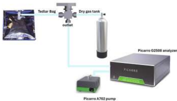
Figure 8.1: Setup to analyze greenhouse gases collected from LUARS.
