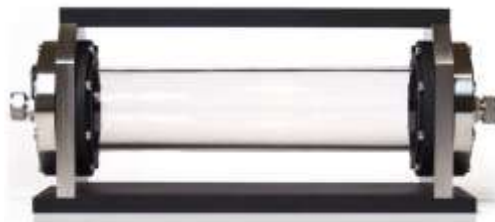
Figure 7.2: Herriot gas cell with 30 m effective path length.
