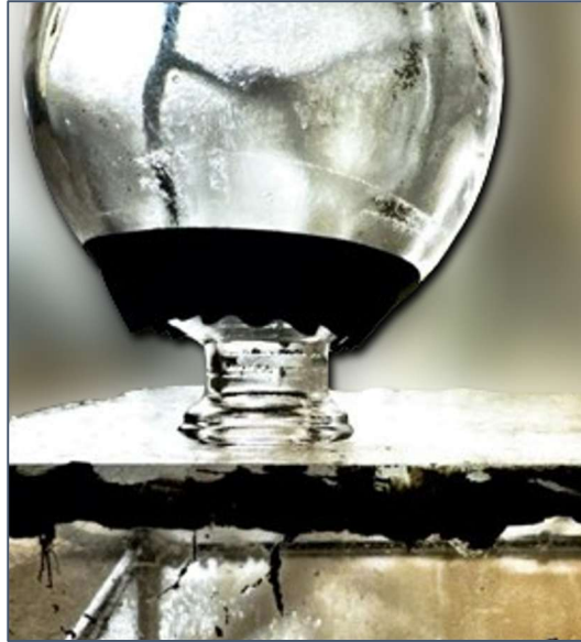
Figure 3.23. Helmholtz resonator with a slit at the neck to house the piezo beam's free end.
