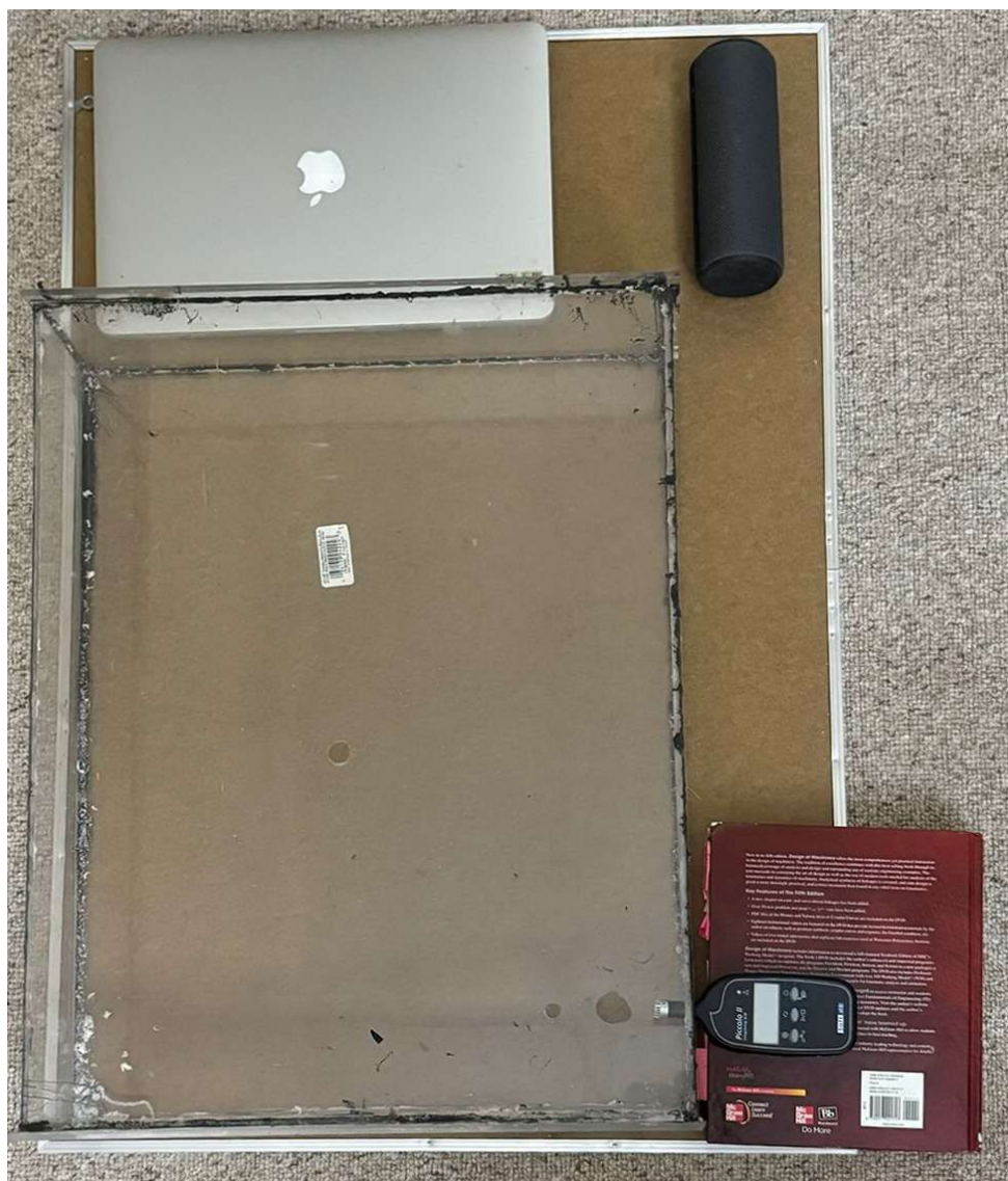
Figure 3.12. The rectangle cavity subject to pink noise and tonal signal from a loudspeaker as measured by a microphone.
