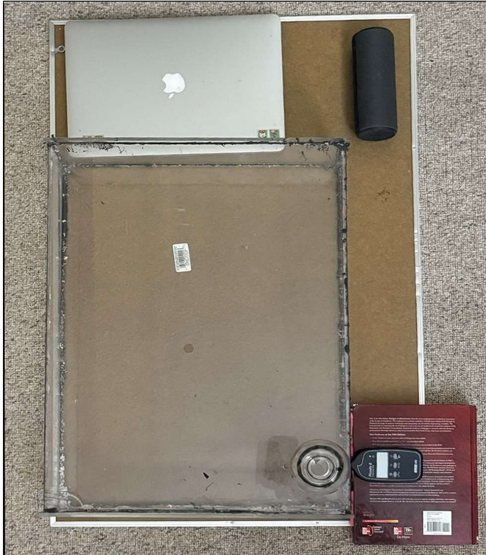
Figure 3.17. The coupled system subject to pink noise and tonal signal from a loudspeaker as measured by a microphone.
