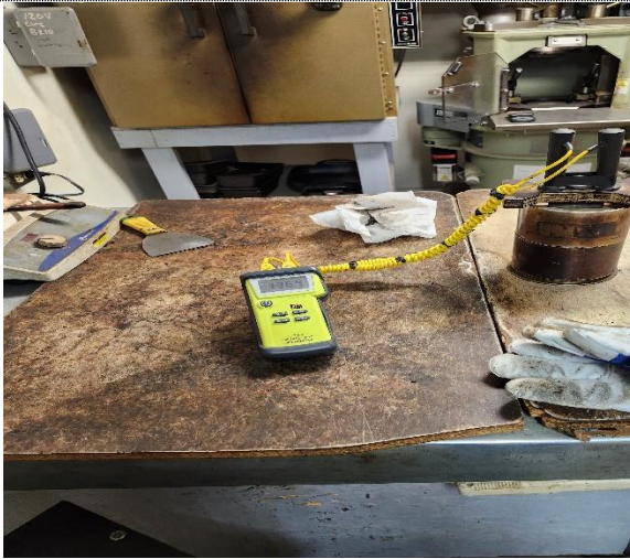
Figure 16: Thermometer inserted to monitor mixture temperature before compaction
