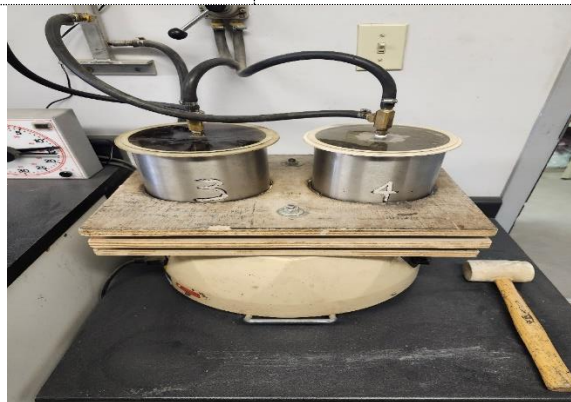
Figure 34: Vacuum saturation of compacted specimens as part of moisture conditioning
