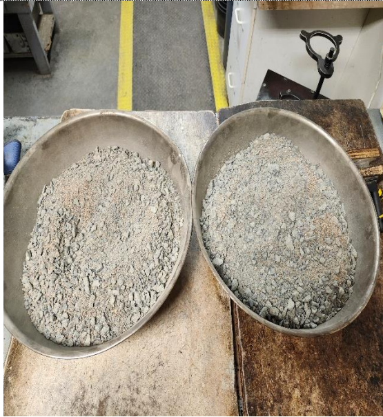
Figure 20: Combined aggregate blend after gradation adjustment, ready for mixing with binder.
