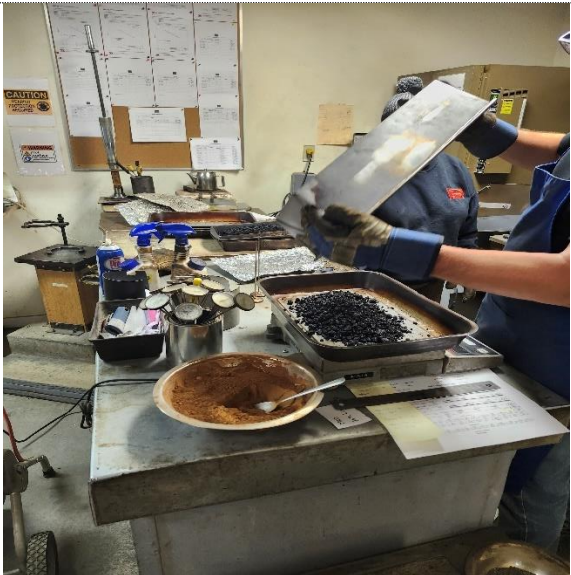
Figure 26: Weighing samples after splitting
