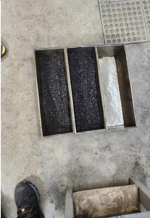
Figure 24: Batched mixtures prepared in trays for short-term aging or compaction.
