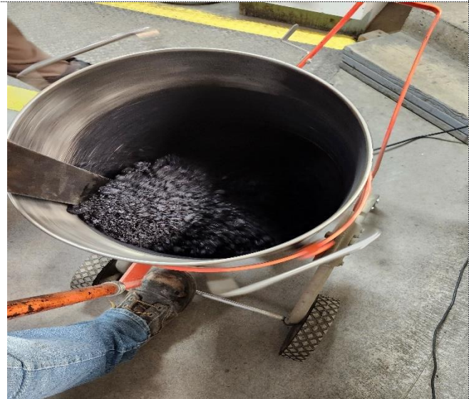
Figure 23: Observation of the homogeneous mixing process of aggregate, bitumen, and lignin
