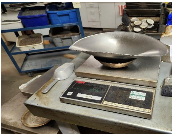
Figure 13: Pan and Scale used for measuring Marshall Samples
