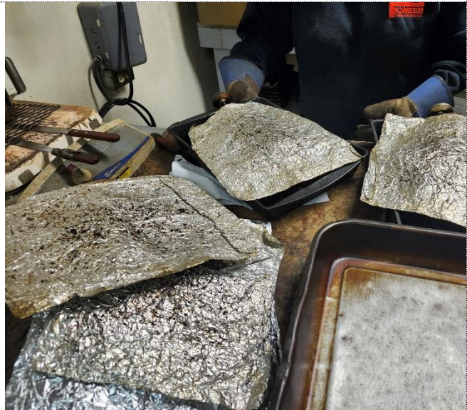
Figure 27: Flattening of hot mix asphalt during tray loading for short-term aging.
