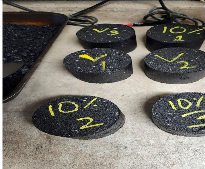
Figure 17:– Compact Marshall specimens labeled for identification based on lignin content.
