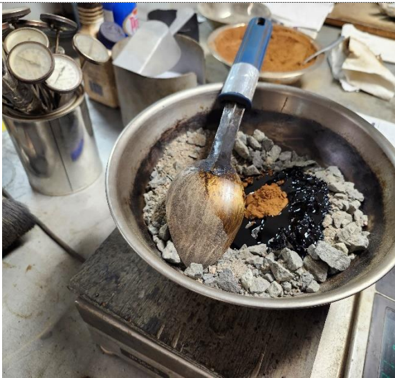
Figure 14: Initial mixing of bitumen, aggregate, and lignin additive for sample preparation
