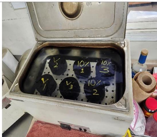
Figure 19: Samples placed in a water bath for temperature conditioning
