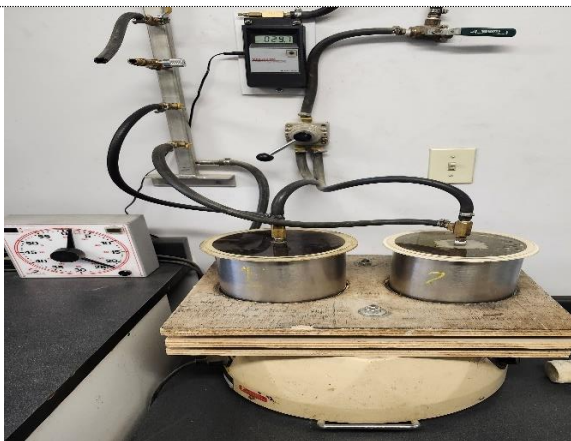
Figure 18: Vacuum saturation of compacted specimens as part of moisture conditioning
