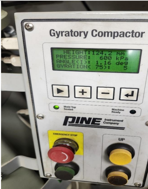
Figure 32: Gyrator Compactor display
