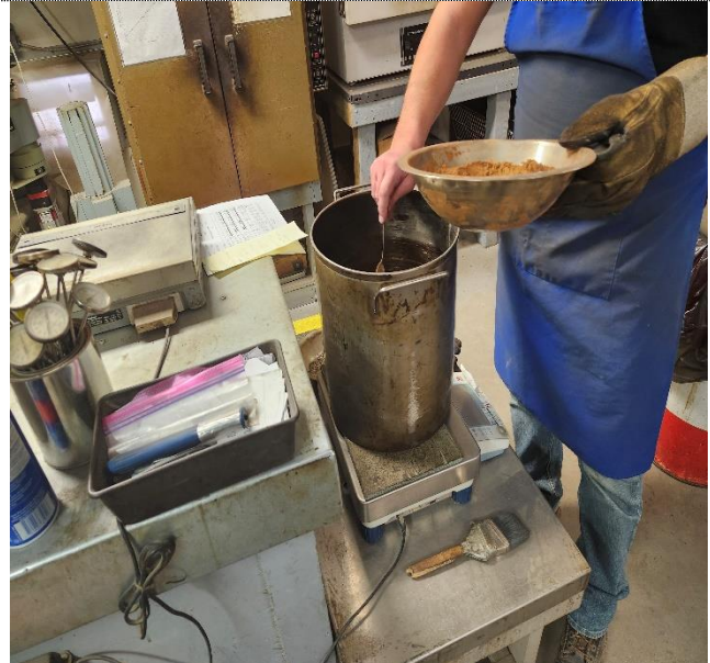
Figure 21: Pouring the bitumen and lignin blend into the mixing bucket for preparation
