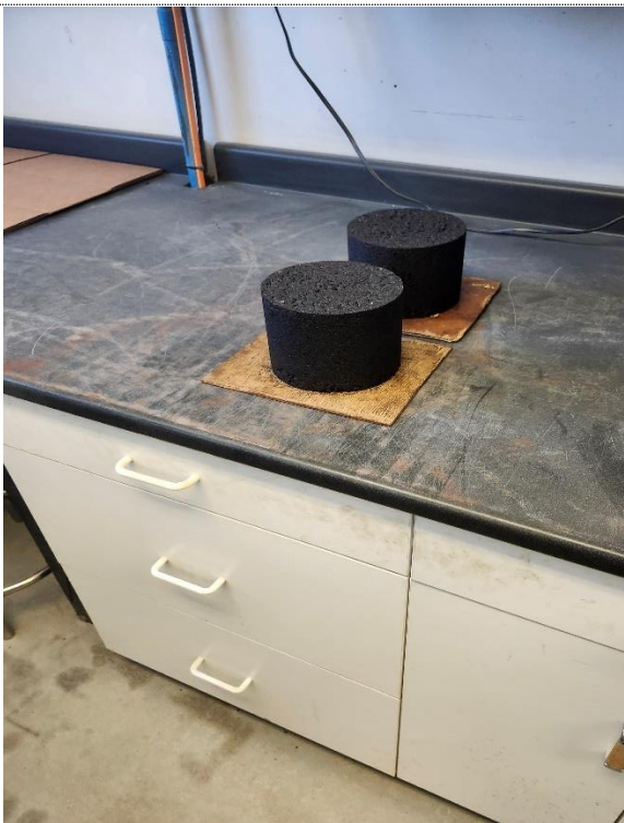
Figure 30: Cooling off molds
