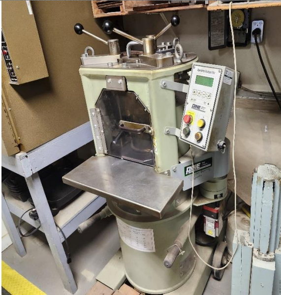
Figure 28: Gyrotory compactor used to compact specimens at N design gyrations under controlled pressure and angle.
