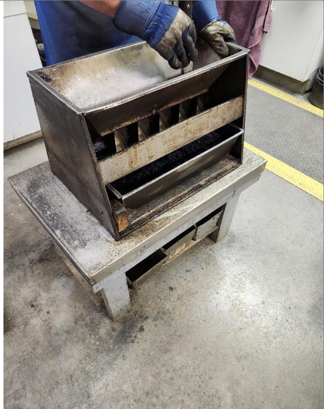
Figure 25: Splitting of the hot-mix asphalt using a mechanical splitter to create consistent sample batches.
