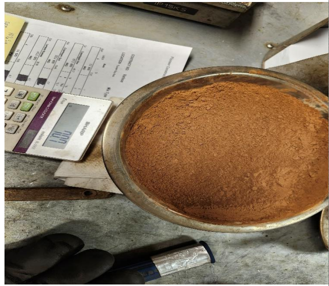
Figure 13: Kraft Lignin provided by FPInnovations
