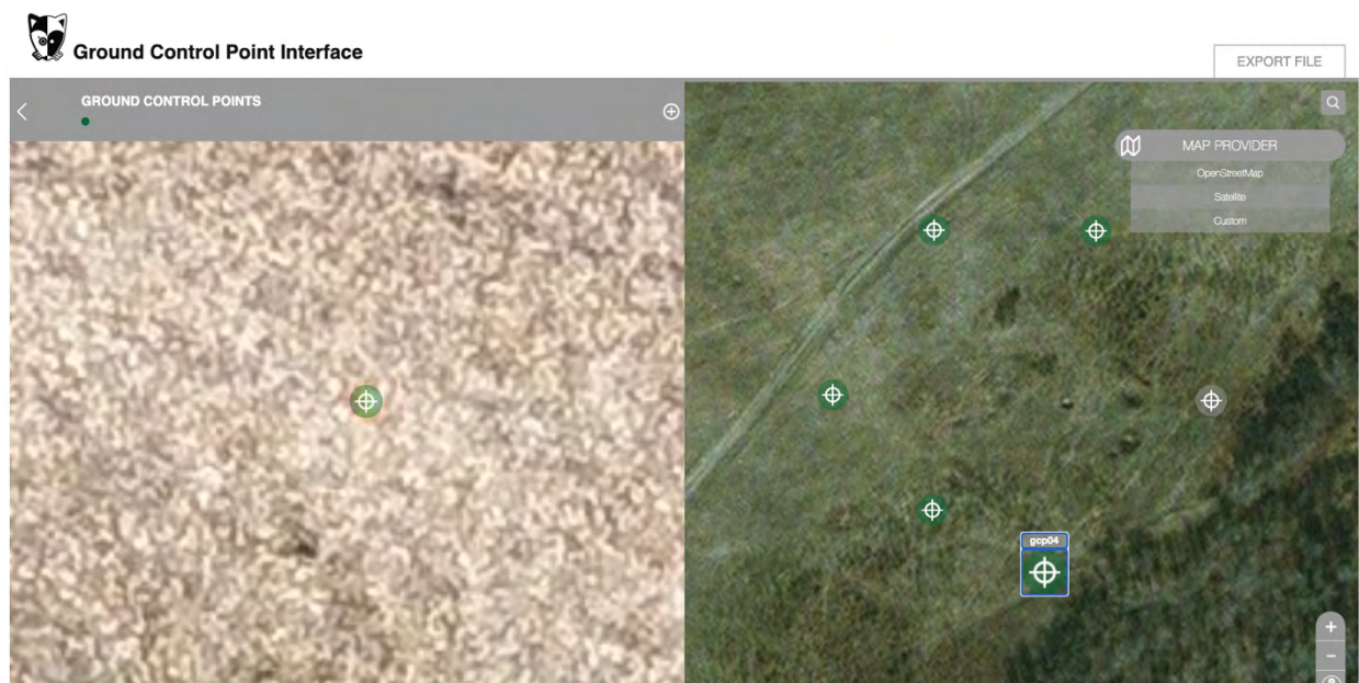
Figure 18. GCP interface in WebODM allowing for PPK
