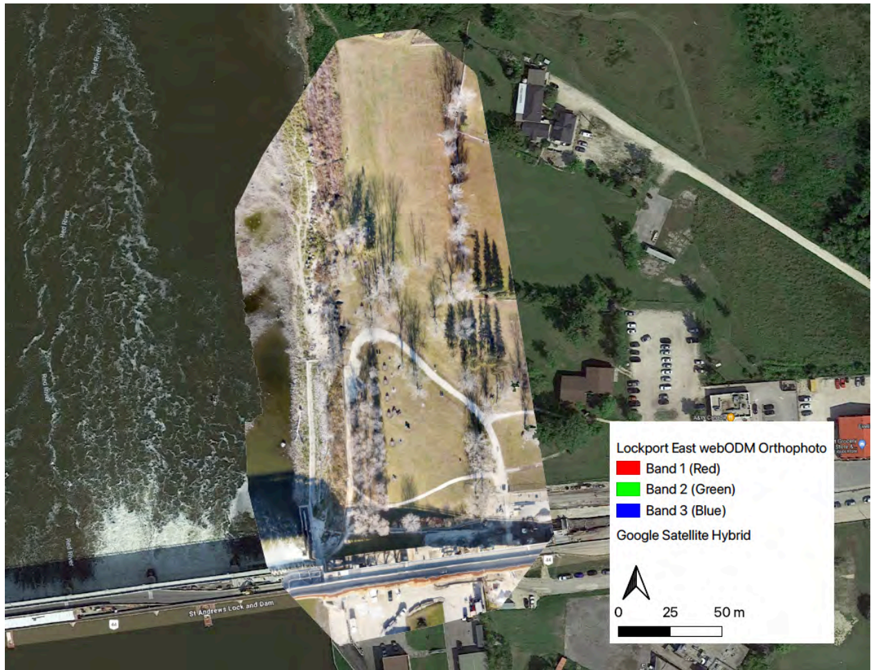
Figure 5. RGB Orthophoto of EaLf-1 captured with a DJI Mavic Mini and processed with WebODM using 'Quick Orthophoto' option.
