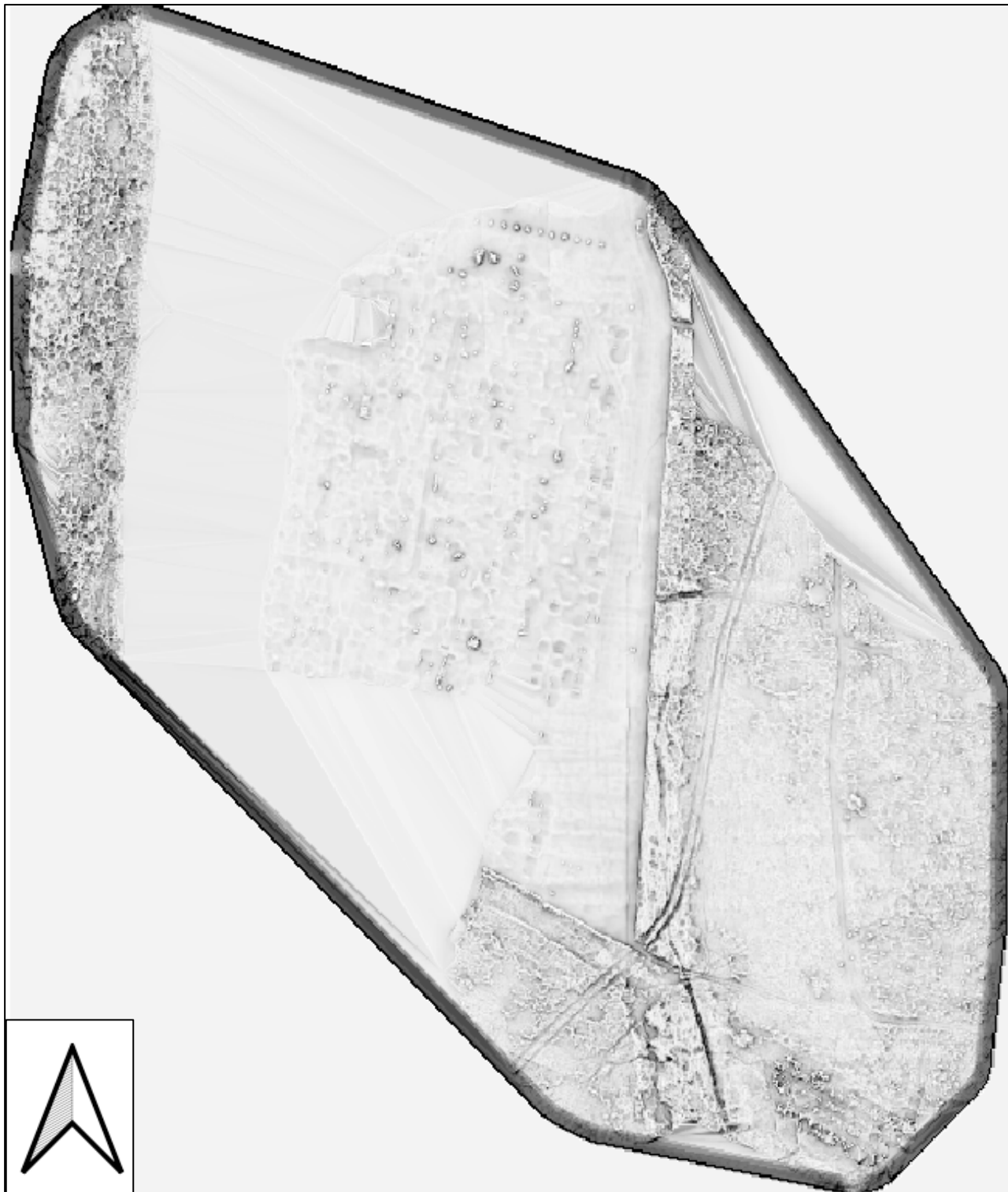
Figure 14. LiDAR VAT model of cemetery built using CloudCompare and GIS software
