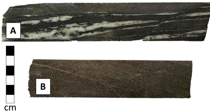
Figure 4.27. Representative core samples of the Quetico metasedimentary rocks. Sample SL23KM01 quartz banding (A). Sample SL23KM40 shows a granular homogeneous composition with a quartz veinlet (B).
