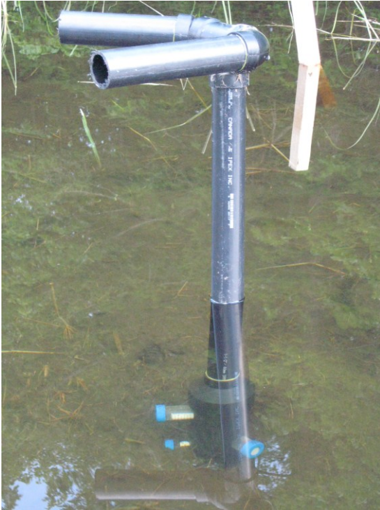
Figure A.4.8 – Marchmont Marsh pore water sampler installed in non-vegetated plot, showing three samplers above sediment-water interface.
