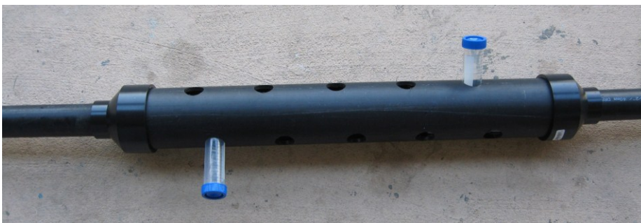
Figure A.4.5 – Completed pore water sampler, showing two installed samplers (all holes filled with samplers during launch).
