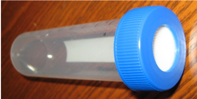
Figure A.4.3 – Constructed pore water sampler.
