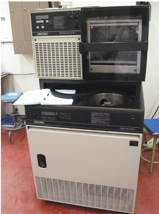
Figure C.5.8 – LABCONCO Freeze Dry System (freeze-dryer) used to dry wild rice root samples. Located in the Lakehead University Instrument Laboratory (LUIL).
