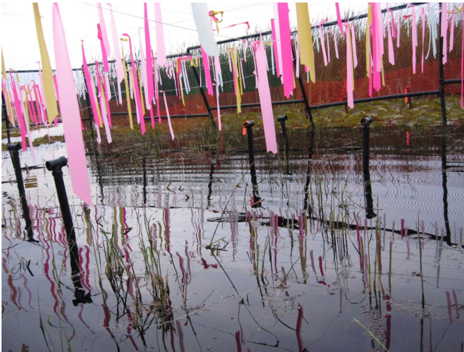
Figure B.4.8 – Victoria Point pore water samplers installed in non-vegetated and vegetated plots.
