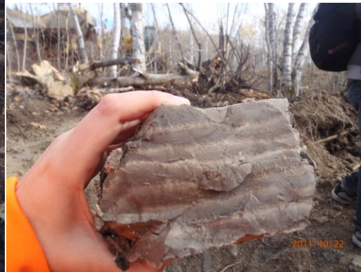
Figure 4.2b and c. Photos of clay bottom found when excavating reach 2 of Kama Creek. Arrow points to thick clay layer in pool of new channel (left). On the right, section of clay showing layering.
