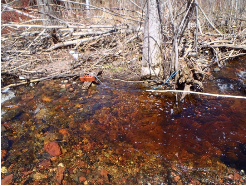
Figure 3.6 Water Temperature Hobo set up and location in reach 2 of Kama Creek.
