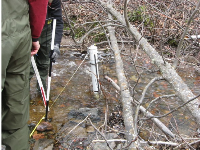
Figure 3.9 Flow meter being used to record velocity in Kama Creek.
