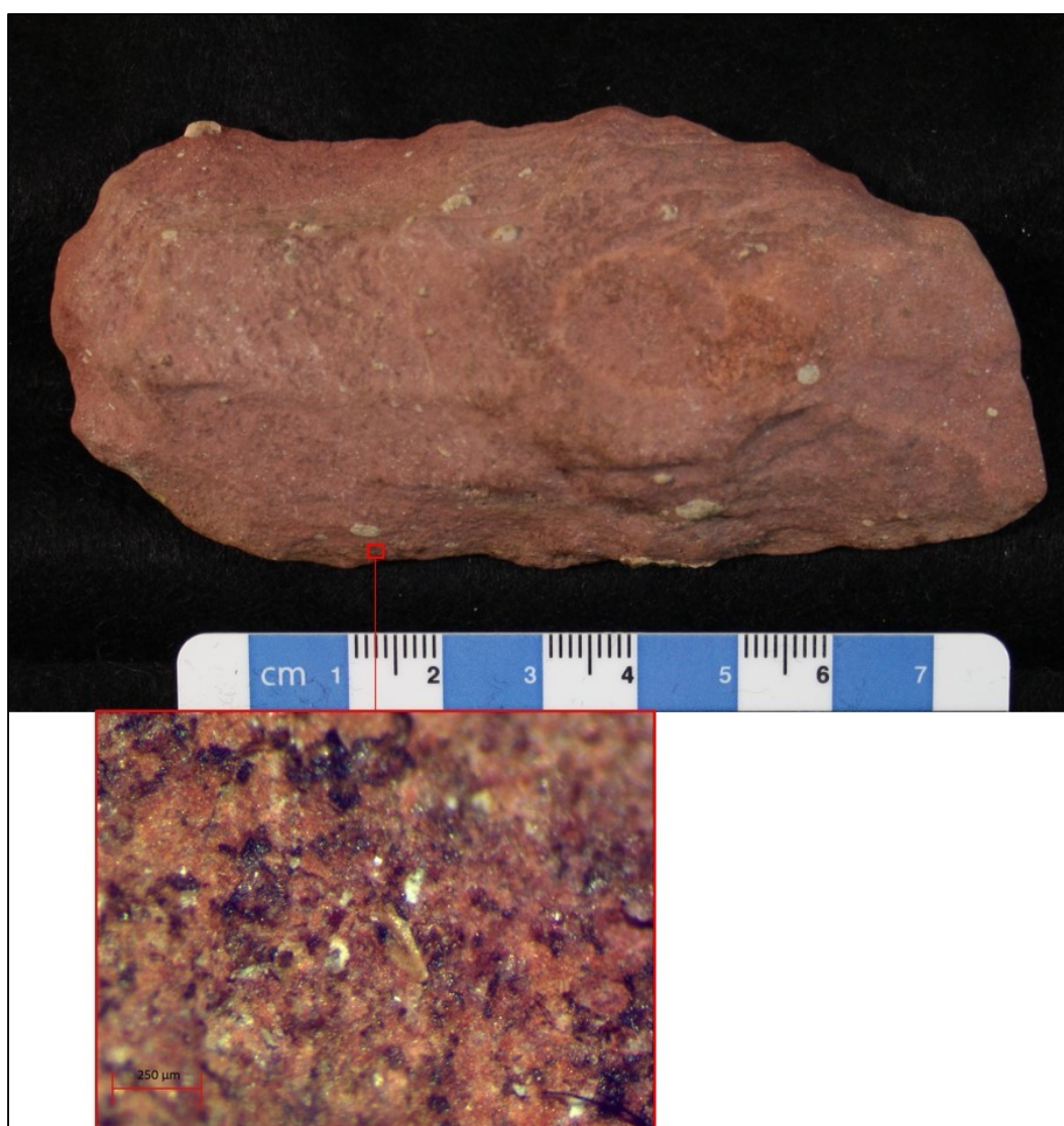
Figure 6.15 Location of dehydroabietic acid identified on artifact DeJj-4(4)
