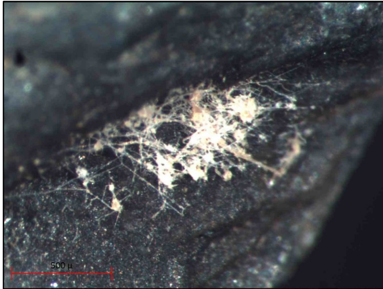
Figure 6.5 White fibrous contamination
