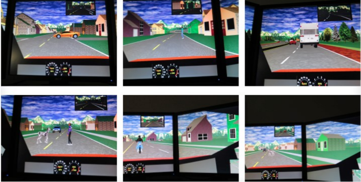
Figure 6. Reaction time scenarios in driving simulation. From top left to bottom right: Vehicle incursion at intersection, pedestrian incursion from side of the road, sudden braking by a vehicle in front of participant, pedestrian incursion in school zone, braking by a vehicle in front of participant, and animal incursion.
