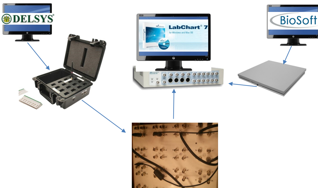
Figure 14. Synchronization of force plate and electromyography data. Reprinted from Trigno Wireless Systems and Smart Sensors, in Delsys, 2016, Retrieved April 4, 2015, from http://www.delsys.com/products/wireless-emg/ .
