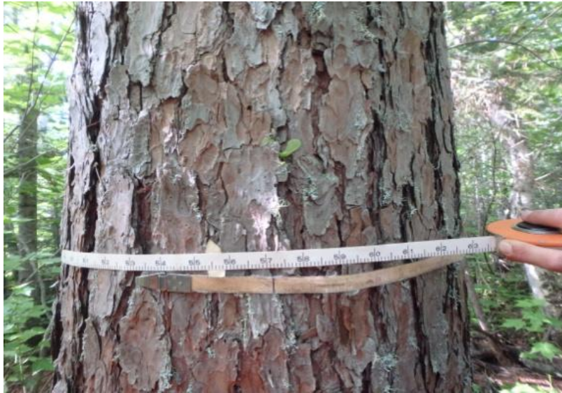
Figure 27. Example of DBH measurement (Seymour 2015).
