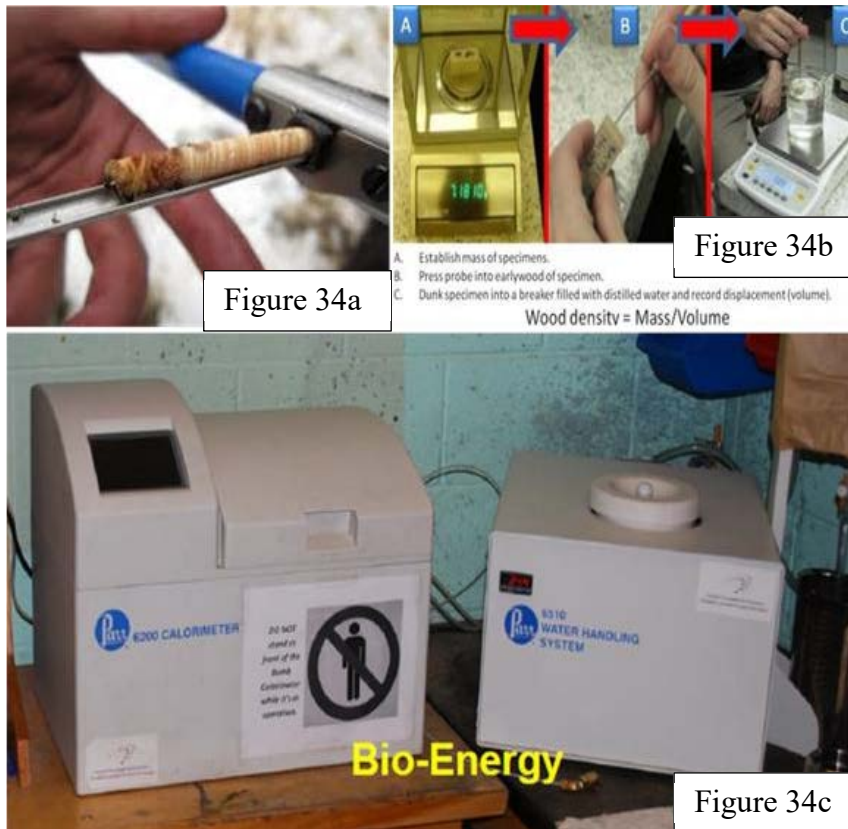
Figure 35. Example of wood properties testing procedures and equipment. Figure 34a. shows the removal of wood from an increment borer. Figure 34b shows the weighing and dunking of wood samples to determine density, and Figure 34c shows the bomb calorimeter where thermal potential is measured.
