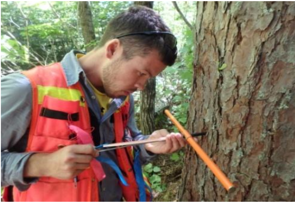
Figure 31. Use of increment borer to determine age (Seymour 2015).
