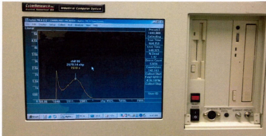
Figure 3.5 The computer is equipped with MCA card and software for analysis and data output. For each PHS experiment, the spectrum can be viewed in real-time which is shown here on the screen.
