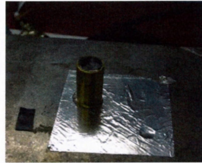
Figure 3.7 The ^{241}\text{Am} source, shielded by lead casing (left) and exposed (right), emits \gamma -rays of 60 keV to the sample for detection. The distance from the source to the detector inside is approximately 5 cm.
