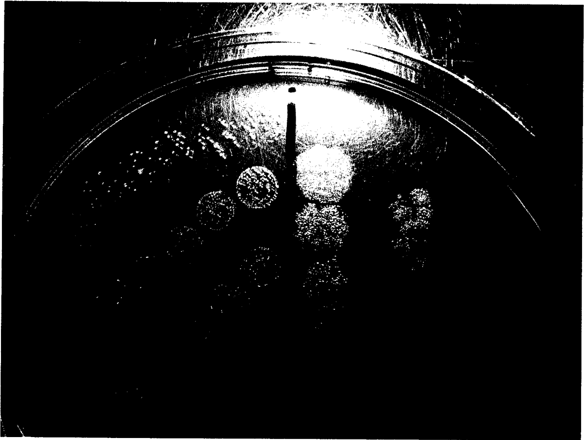
Figure 5.31 - Contamination in effluent of silt columns. Column silt R (left) contained minimal contamination, while column Silt S (right) could not be analyzed for E. coli colonies due to extensive contamination.
