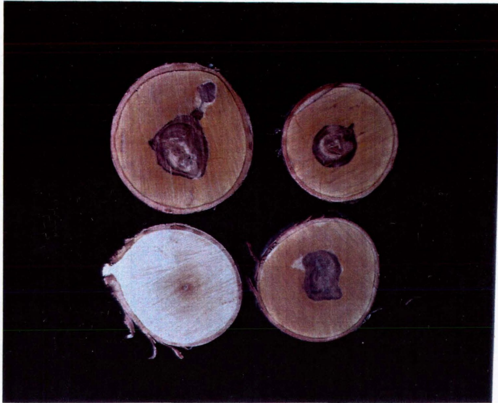
Figure 3.2. Typical examples of "red heart" discolouration and clear wood in paper birch.
