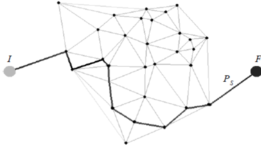
Figure 2.2-4 Sensory Field with Weighted Delaunay Triangulation and Maximal Support Path ( P_s )
