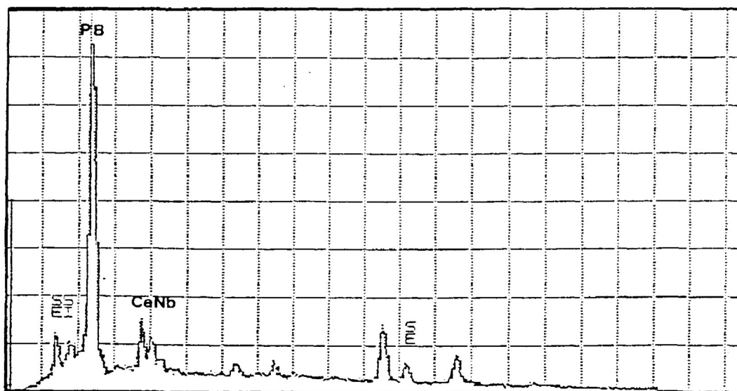
Figure 3.22 The spectrum of clausthalite (PbSe) which occurs adjacent to a Ce-Nb mineral. Sample G-46.
