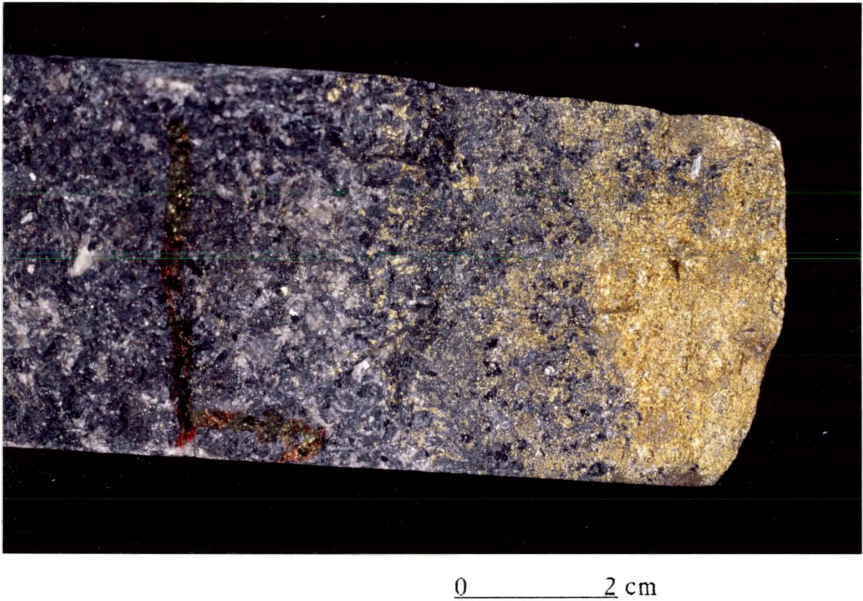
Figure 3.1 The style of chalcopyrite mineralization (bright yellow) in a core slab from core 3 of the GLI, showing a gradual increase of the Cu-sulphide concentration from a few specks to massive aggregates. The host rock is an ophitic olivine gabbro (sample G-309).
