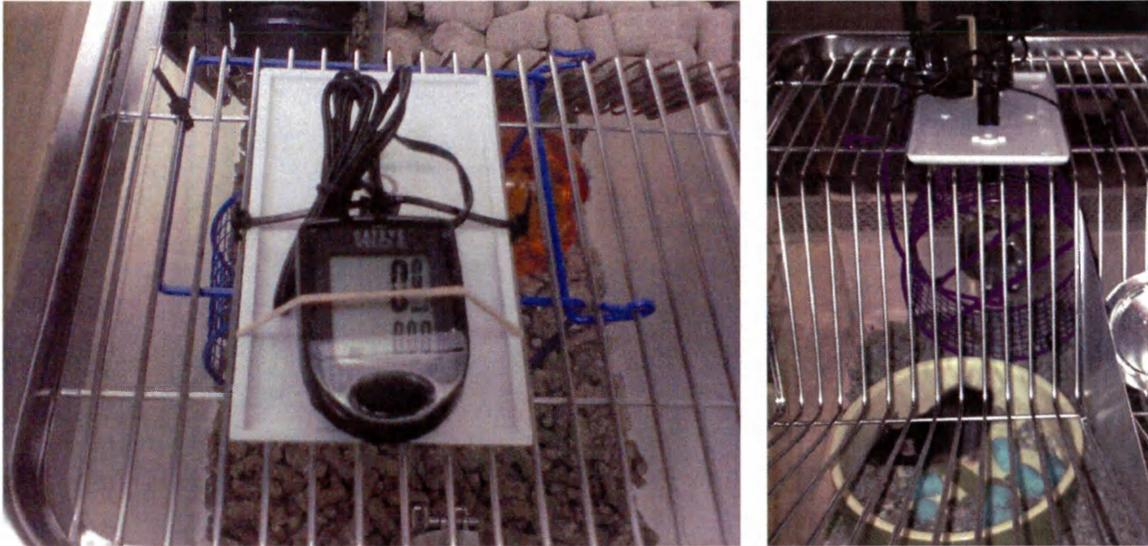
Running wheels (4.5 inch Run Around Wheels) were suspended from the top of the cage. A magnet was attached to the running wheel, and the CatEye Velo 5 sensor was suspended through a light switch cover. The purpose of the light switch cover was to prevent the mice from chewing on the wires. The CatEye Velo 5 sensor tracked wheel revolutions, and distance was adjusted based on wheel circumference.
