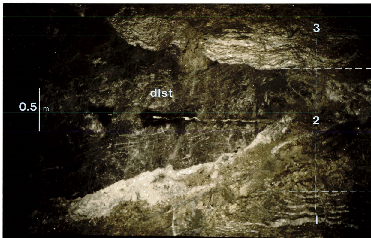
FIGURE 1.12 - COARSELY BANDED ORE FROM UNIT 1 IN CONTACT WITH AN OVERLYING DOLOSTONE FIN. UNITS 2 AND 3 ALSO INDICATED.
