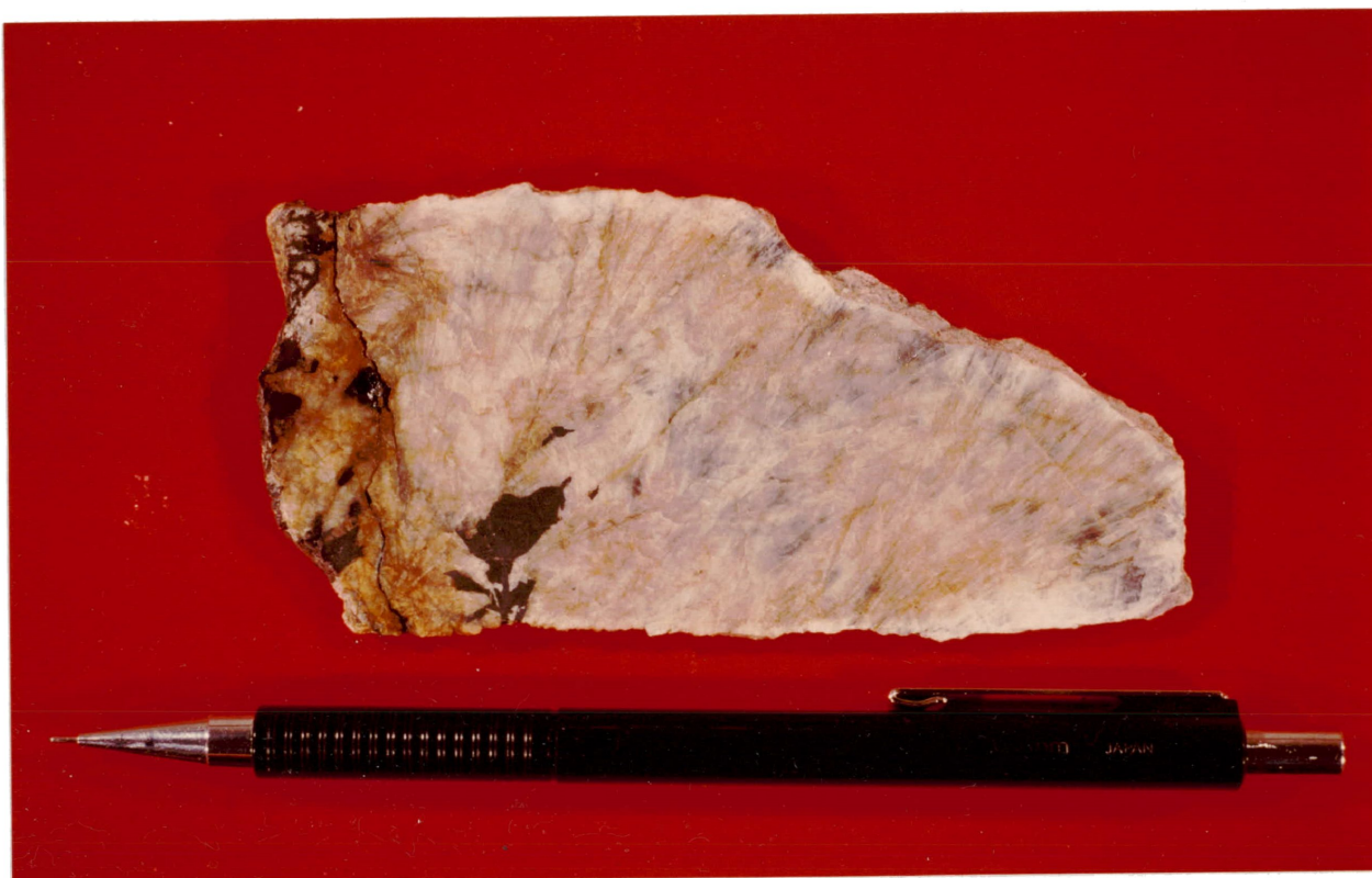
Fig. 3-6. Sn oxide minerals with ferrocolumbite-ferrotantalite inclusions (black) in cleavelandite; intermediate zone, MNW pegmatite.
