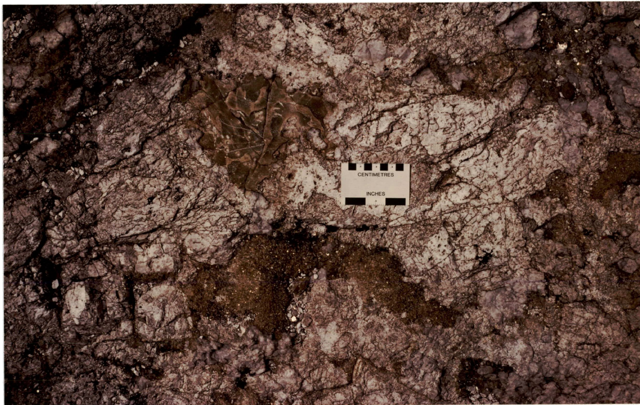
Fig. 3-12. Podiform green microcrystalline muscovite (above and left of scale bar) and fine-grained green muscovite (below scale bar) replacing perthitic microcline; Brink pegmatite.
