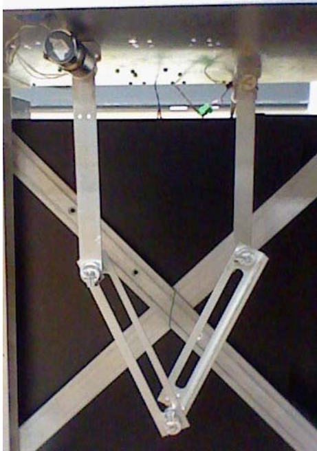
Figure 6.7: Close-up View of the Two Degrees of Freedom Parallel Robot
