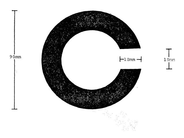
Each figure is constructed so that the thickness of the line segment is one-fifth the height of the 'C' and equal to the gap.
