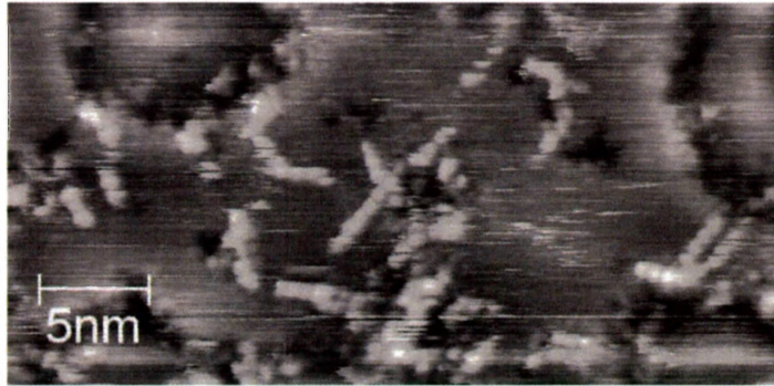
Figure 4.3. An STM image of 1-d TBTTA islands on the \sqrt{3} surface ( U_{\text{bias}} = 1.89 V, I_{\text{tunnel}} = 257 pA; 350 \text{ \AA} \times 170 \text{ \AA} ).
