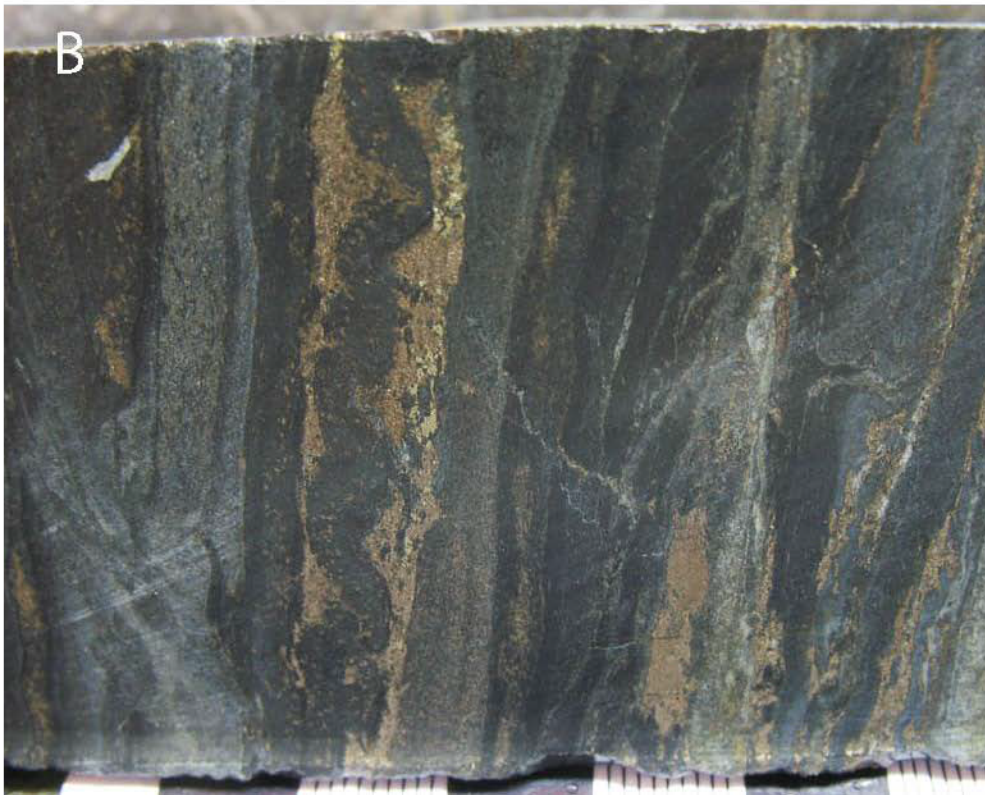
Figure 4.10 – A.) Magnetite discrimination diagram based off Beaudoin and Dupuis, 2010, B.) Wispy banded pyrrhotite from drill core, dark bands are magnetite and wispy brown mineral is pyrrhotite.
