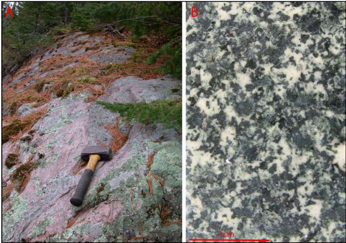
Figure 3.6 – A.) Outcrop of the Powell Lake granite on the western shore of Hamlin Lake, and B.) Fine grained “gabbro” intersected in hole HAM09-59, the mafic minerals are largely altered to chlorite and biotite.
