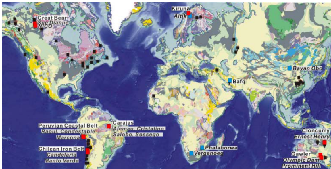
Figure 1.1 – Global distribution of IOCG deposits. Red squares are IOCG deposits, black squares are IOCG occurrences and blue squares are IOCG-like occurrences. Districts are named on a white background (from Corriveau and Mumin, 2009).
