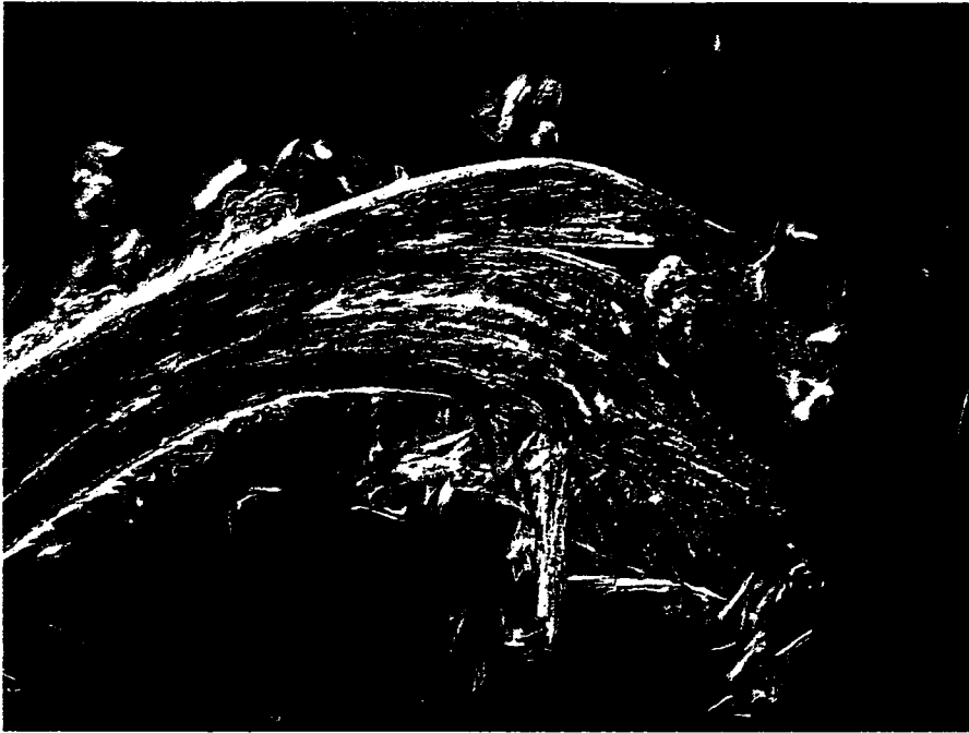
Figure 5. Differential Interference Contrast micrograph of frayed hair shaft. Many cuticular cells have separated from the cortex. Bundles of cortical cells (~100 \mu\text{m} in length) are visible. The hair shaft is ~87 \mu\text{m} wide.
