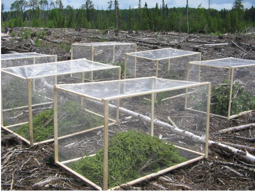
Figure 4. Typical arrangement of the netted biomass enclosures at a site.
