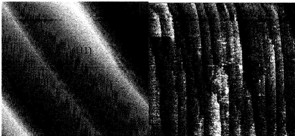
Figure 2-1-6 (a) An STM image ( 2000 \text{ \AA} \times 1800 \text{ \AA} ) of a 3.8^\circ clean surface taken at a bias of +2.32 V, tunneling current of 29.0 pA, with a PtRh tip. (b) An STM image ( 3000 \text{ \AA} \times 3000 \text{ \AA} ) of a clean 12.3^\circ surface taken at a bias of +2.42 V, tunneling current of 323 pA, with a PtRh tip.
