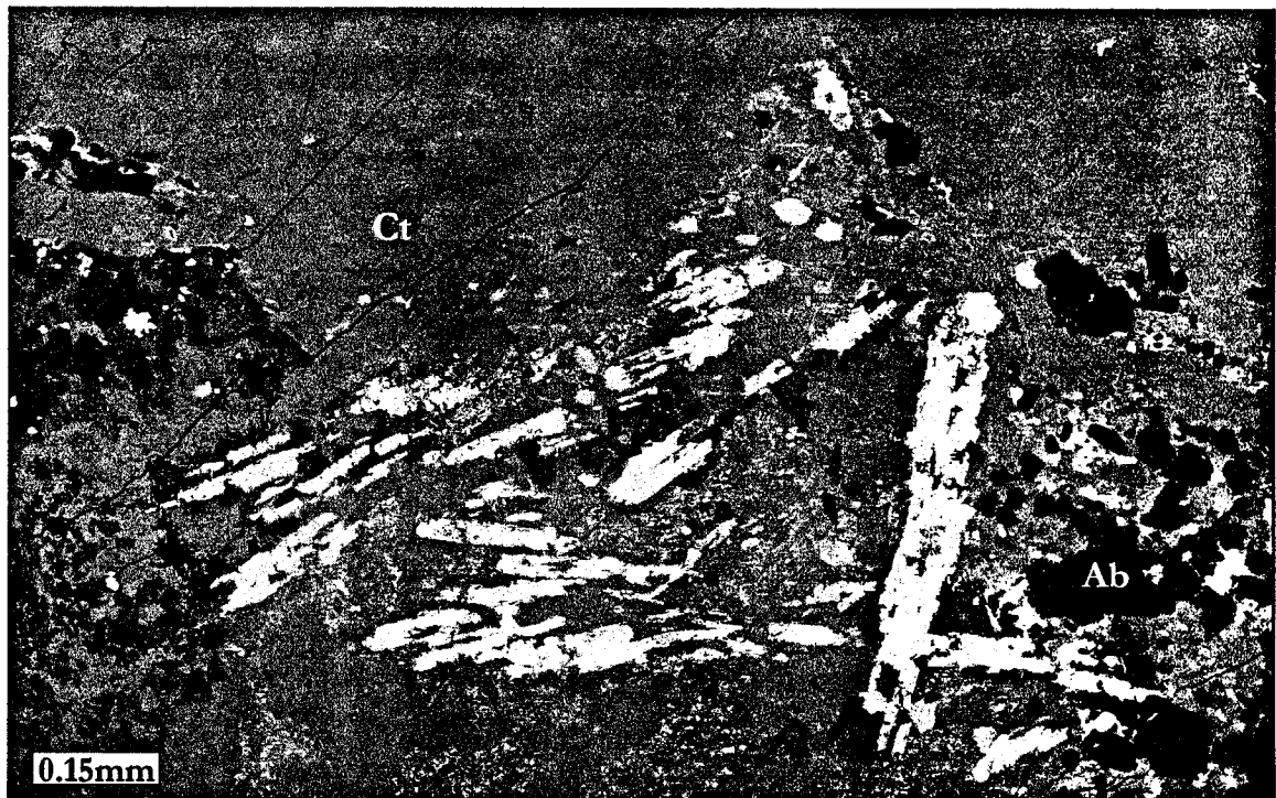
Figure 2.55: BSE-image of corroded and altered rutile laths set in a calcite (Ct) plus albite (Ab) groundmass. White blebs are hematite grains.
