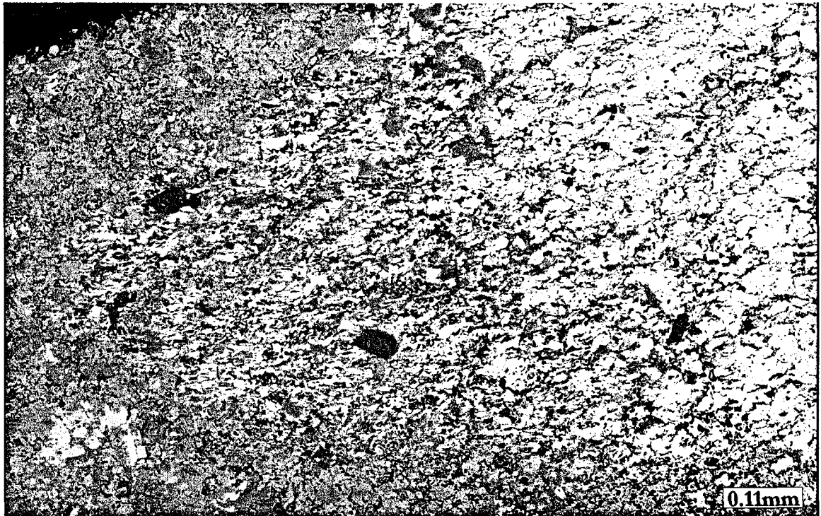
Figure 3.7: BSE-image of the barian feldspars (white) set in a potassium feldspar and augite groundmass.
