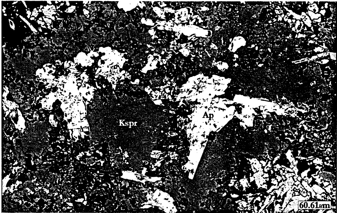
Figure 3.3: BSE-image of subhedral apatite (Ap) and aegirine-augite (Ae) set in potassium feldspar (Kspr).
