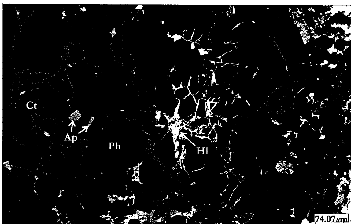
Figure 2.31: BSE-image of hollandite (Hl), calcite (Ct) and apatite grains (Ap) interstitial to large phenakite grains (Ph).
