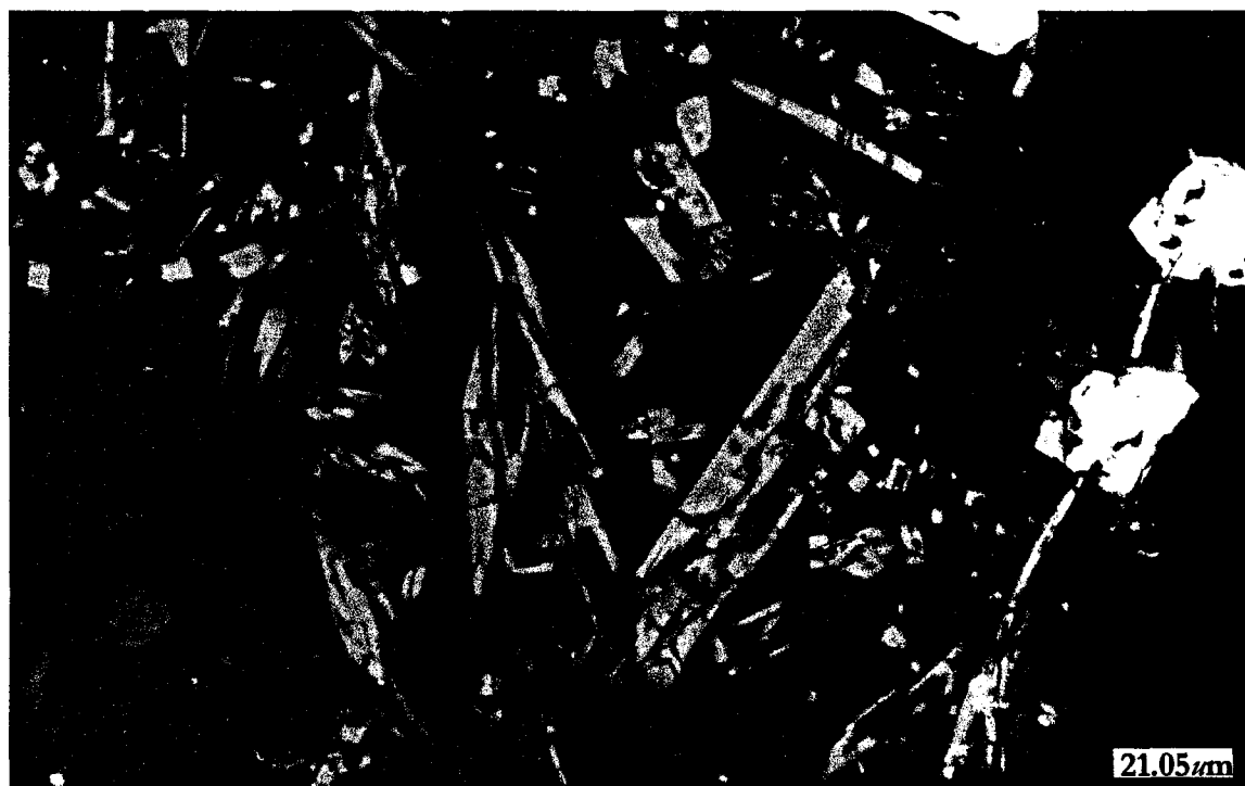
Figure 2.44: BSE-image of aegirine-natalyite grains and the hydrated calcium zirconosilicate set in quartz.
