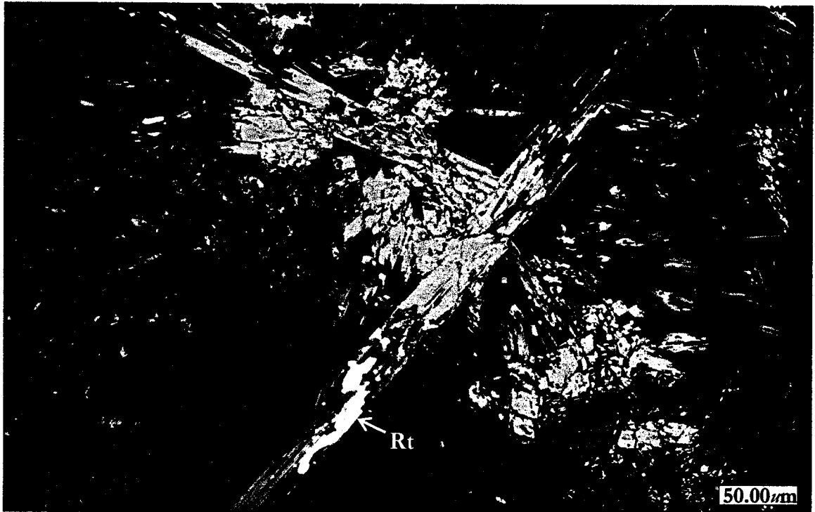
Figure 2.45: BSE-image of aegirine-natalyite grains set in quartz, with accessory subhedral rutile (Rt).
