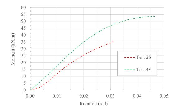
Figure 4.4 Moment-rotation relationships of test assemblies 2S and 4S using six bolts with four and five-times bolt dia. end distance, respectively.
