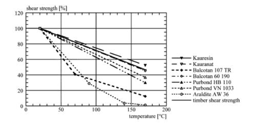
Figure 2.29 Shear strength reduction with respect to change in temperature (Adapted from Frangi et al., 2004).
