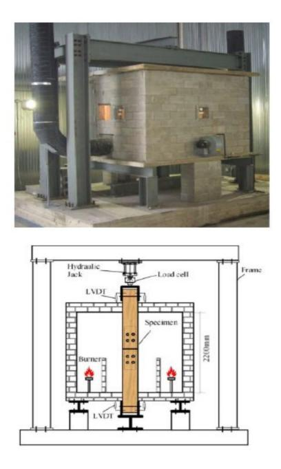
Figure 2.32 Test furnace at Carleton University's Fire Lab (above), Test set-up (below). (Adapted from Peng et al., 2012).
