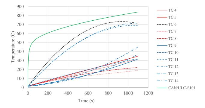
(b) Test 2FS (six-bolt strengthened connection with four-times bolt diameter end distance).
