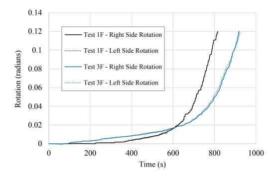
Figure 5.1 Time-rotation relationships developed to illustrate the effect of changing the bolt end distance in fire resistance Tests 1F and 3F, both with four bolts.
