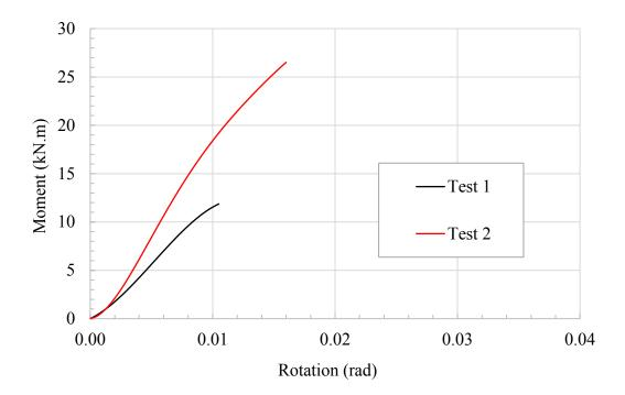
Figure 4.5 Moment-rotation relationships of test assemblies 1 and 2 using four and six bolts with four-times bolt dia. end distance, respectively.
