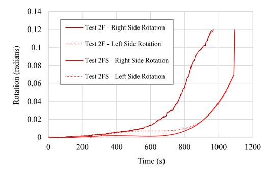
Figure 5.10 Time-rotation relationship showing the effect of perpendicular STS strengthening on the rotational resistance of connections with six bolts and four-times bolt end distance.
