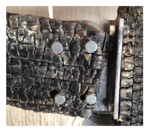
Figure 5.18 Failure modes observed in STS-strengthened connection with four bolts and fivetimes bolt diameter end distance (hole elongation, reduced brittle failure modes and complete combustion of almost all wood between the face and the first column of bolts)
