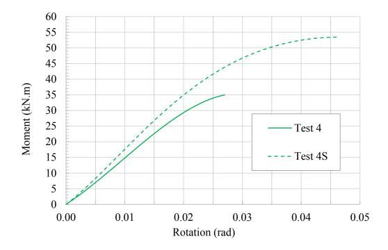
Figure 4.12 Moment-rotation relationships for assemblies in test groups 4 and 4S using six bolts and five-times bolt dia. end distance, unstrengthened vs. strengthened, respectively.
