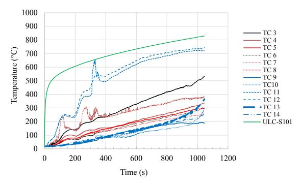
(d) Test 4F (six-bolt connection with five-times bolt diameter end distance).Figure 5.13 Actual time-temperature curves of all thermal measurements taken in fire resistance Tests 1F through 4F.
