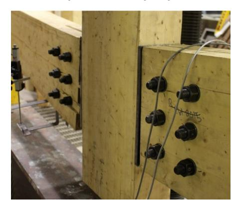
Figure 3.9 A general beam-to-column test assembly with six steel bolts in three rows.
