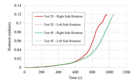
Figure 5.2 Time-rotation relationships developed to illustrate the effect of changing the bolt's end distance in fire resistance Tests 2F and 4F, both with six bolts.
