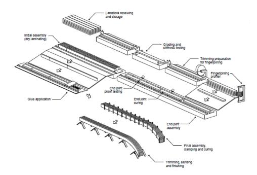
Figure 2.2 Typical glulam manufacturing process (Adapted from Canadian Wood Council, 2010).
