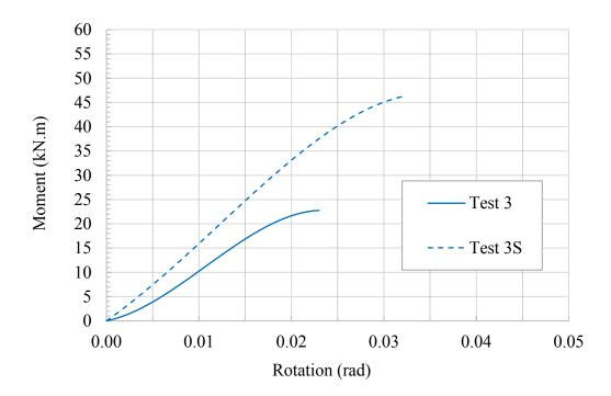
Figure 4.11 Moment-rotation relationships for assemblies in test groups 3 and 3S using four bolts and five-times bolt dia. end distance, unstrengthened vs. strengthened, respectively.
