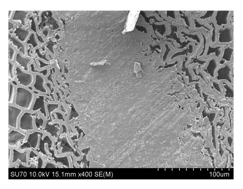
Figure 2.22 Glulam SEM cross section with glue line details.
