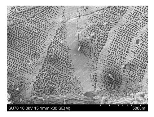
Figure 2.21 Glulam SEM cross section overview.
