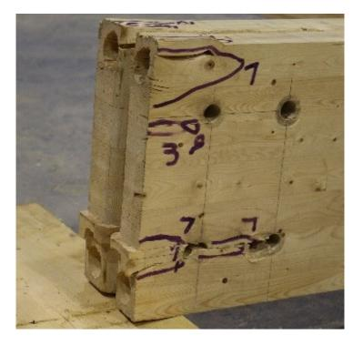
(a) Brittle failure modes in Test 1S with four bolts and four-times bolt diameter end distance.
