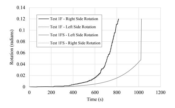
Figure 5.9 Time-rotation relationship showing the effect of perpendicular STS strengthening on the rotational resistance of connections with four bolts and four-times bolt end distance.
