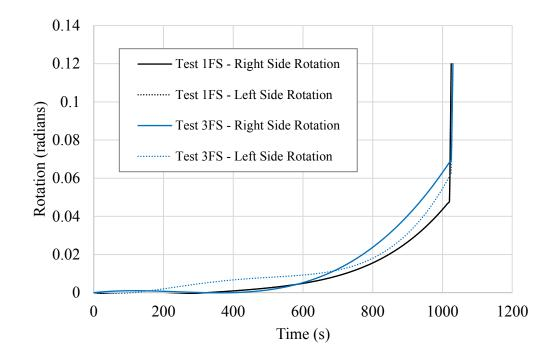
Figure 5.3 Time-rotation relationships developed to illustrate the effect of changing the bolt's end distance in fire resistance Tests 1FS and 3FS, both with four bolts.
