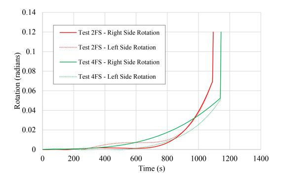
Figure 5.4 Time-rotation relationships developed to illustrate the effect of changing the bolt's end distance in fire resistance Tests 2FS and 4FS, both with six bolts.
