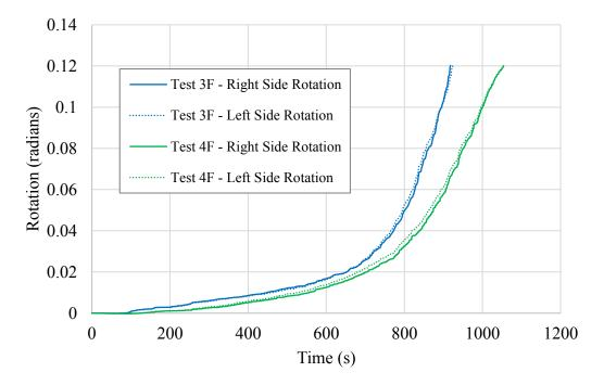
Figure 5.6 Time-rotation relationships developed to illustrate the effect of changing the number of bolts in fire resistance Tests 3F and 4F, both with five-times bolt end distance
