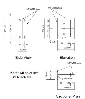
(b) Steel T-stub connector with five-times bolt diameter end distance.
