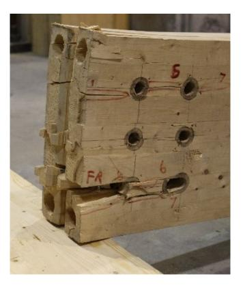
(b) Brittle failure modes in Test 4S with six bolts and five-times bolt diameter end distance.
