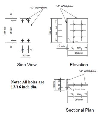
(a) Steel T-stub connector with four-times bolt diameter end distance.
