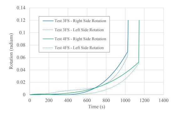
Figure 5.8 Time-rotation relationships developed to illustrate the effect of changing the number of bolts in fire resistance Tests 3FS and 4FS, both with five-times bolt end distance.
