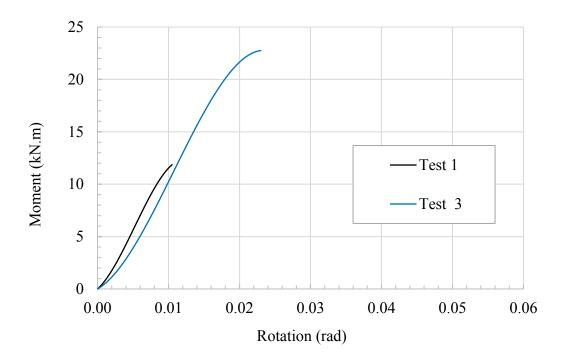
Figure 4.1 Moment-rotation relationships of test assemblies 1 and 3 using four bolts with four and five-times bolt dia. end distance, respectively.
