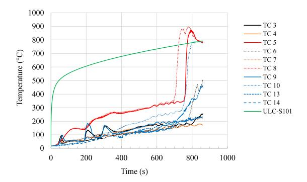
(a) Test 1F (four-bolt connection with four-times bolt diameter end distance).
