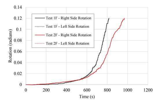
Figure 5.5 Time-rotation relationships developed to illustrate the effect of changing the number of bolts in fire resistance Tests 1F and 2F, both with four-times bolt end distance.
