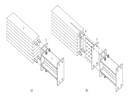
Figure 2.25 Steel-timber connection (a) without, and (b) with glued-in steel plate (Adapted from Andreolli et al., 2011)
