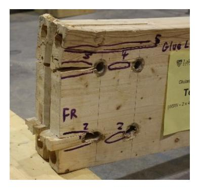
b) Brittle failure modes in Test 3S with four bolts and five-times bolt diameter end distance
