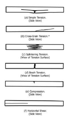
Figure 2.11 Wood failure modes in static bending (Adapted from ASTM, 2016).
