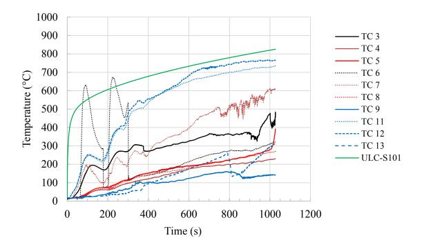
(b) Test 2F (six-bolt connection with four-times bolt diameter end distance).
