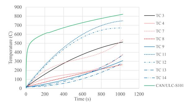
(c) Test 3FS (four-bolt strengthened connection with five-times bolt diameter end distance).
