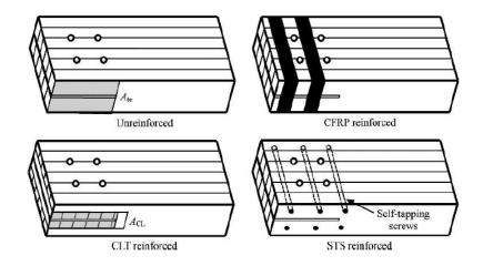
Figure 2.39 Concealed moment-resisting connection strengthening methods (Adapted from Song et al., 2016).
