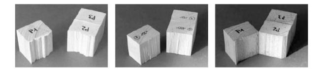
Figure 2.30 Failure Modes: timber outside of bond line (left), failure between wood and bond line (center), and failure of glue cohesion (right) (Adapted from Frangi et al., 2004).
