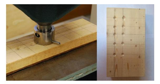
Figure 2.12 Janka-ball hardness test (Courtesy of Dr. Leitch, 2015).
