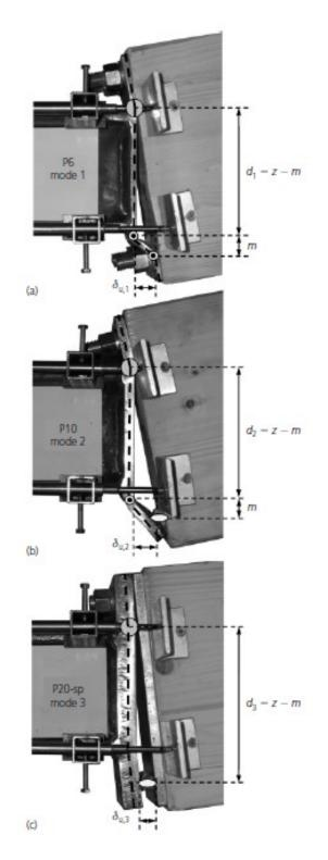
Figure 2.26 Failure modes observed: (a) Complete yielding in flange; (b) bar failure and flange yielding; (c) bar failure (Adapted from Andreolli et al., 2011).
