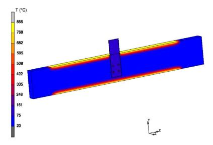
Figure 2.36 FEM verifying temperature distribution observed during experimental trials. (Adapted from Martin and Tingley, 2000).
