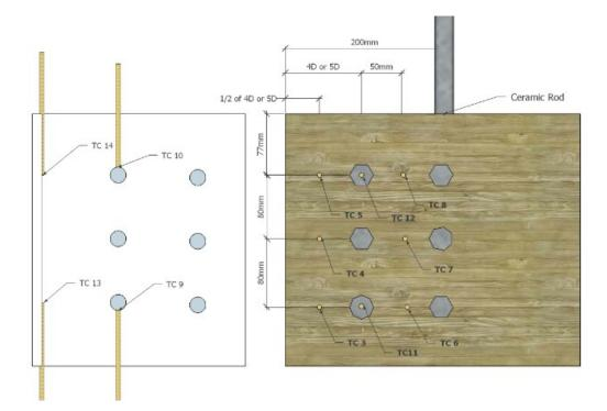
Figure 3.12 Thermocouples layout, steel plate left and wood beam right.
