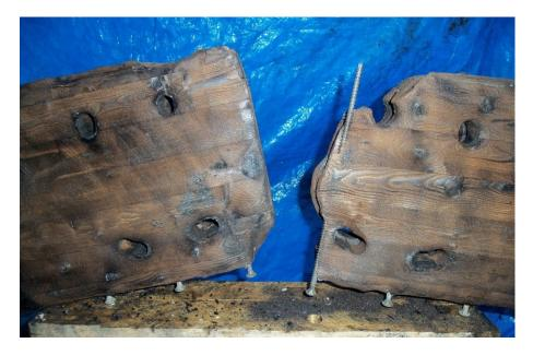
(c) Charred layer removed from Test 3FS assembly (four-bolt strengthened connections with five-times bolt diameter end distance).
