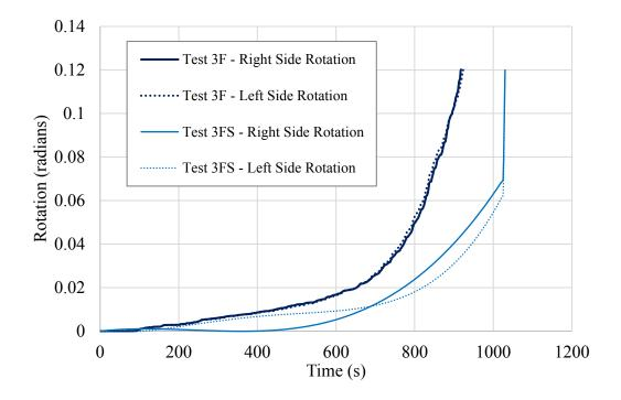
Figure 5.11 Time-rotation relationships showing the effect of perpendicular STS strengthening on the rotational resistance of connections with four bolts and five-times bolt end distance.
