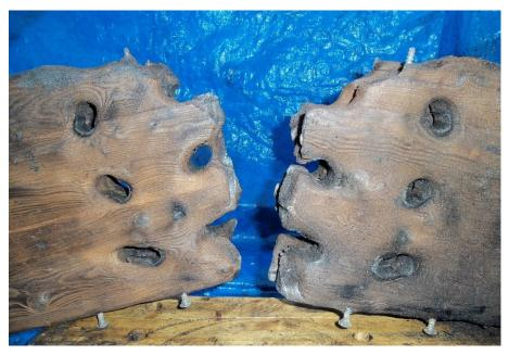
(b) Charred layer removed from Test 2FS assembly (six-bolt strengthened connections with four-times bolt diameter end distance).
