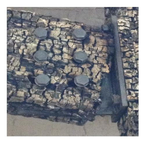
Figure 5.19 Failure modes observed in STS-strengthened connection with six bolts and fourtimes bolt diameter end distance (increased hole elongation and reduced brittle failure modes)
