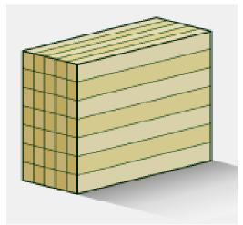
Figure 2.1 Nordic Lam, glulam cross-section (Adapted from Nordic, 2016).
