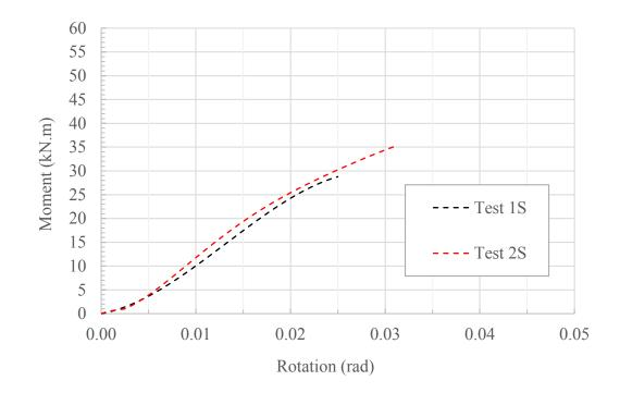
Figure 4.7 Moment-rotation relationships of test assemblies 1S and 2S using four and six bolts with four-times bolt dia. end distance, respectively (both STS-strengthened).
