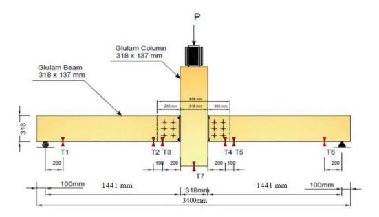
Figure 3.10 Test setup and dimensions of a general glulam beam-to-column test assembly.
