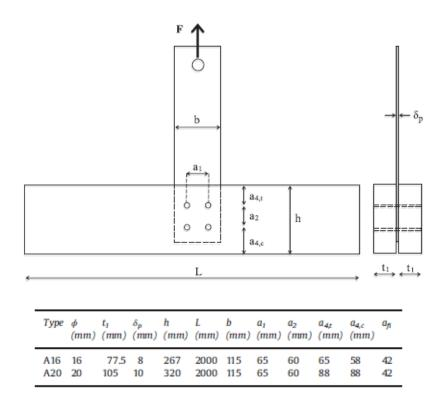
Figure 2.34 Geometric configuration WSW (Adapted from Audebert et al., 2014).
