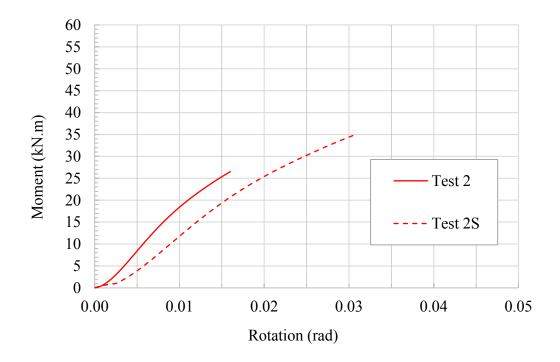
Figure 4.10 Moment-rotation relationships for assemblies in test groups 2 and 2S using six bolts and four-times bolt dia. end distance, unstrengthened vs. strengthened, respectively.
