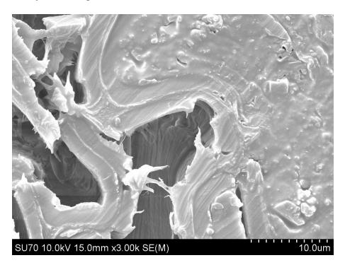
Figure 2.24 Glulam SEM cross section, glue-wood bond and interface details.
