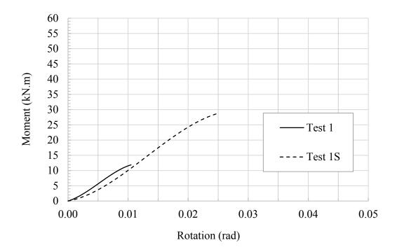
Figure 4.9 Moment-rotation relationships for assemblies in test groups 1 and 1S using four bolts and four-times bolt dia. end distance, unstrengthened vs. strengthened, respectively.
