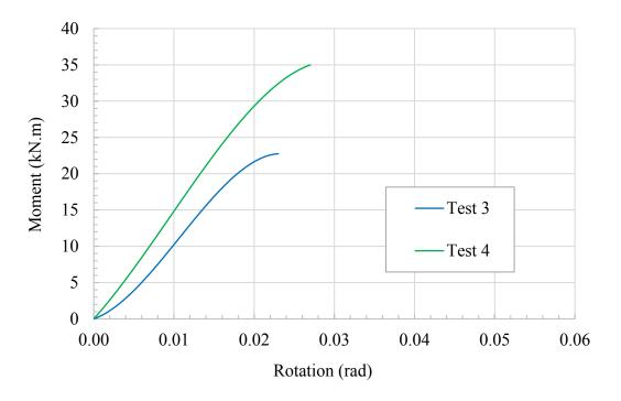
Figure 4.6 Moment-rotation relationships of test assemblies 3 and 4 using four and six bolts with five-times bolt dia. end distance, respectively.
