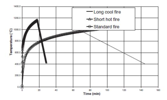
Figure 2.38 Three fire scenarios developed for fire testing (Adapted from Lamont et al., 2006).
