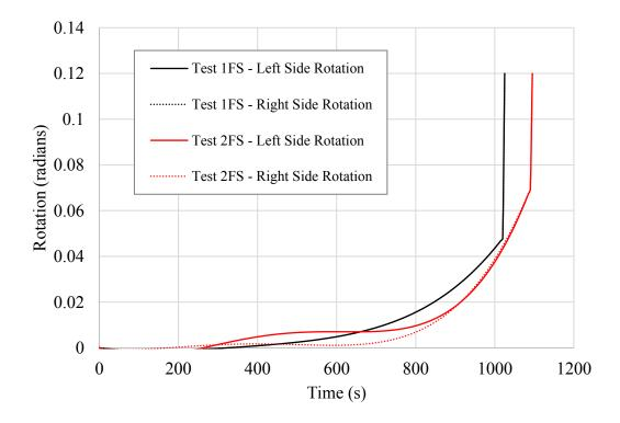
Figure 5.7 Time-rotation relationships developed to illustrate the effect of changing the number of bolts in fire resistance Tests 1FS and 2FS, both with four-times bolt end distance.
