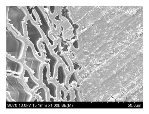
Figure 2.23 Glulam SEM cross section with glue-wood line details.
