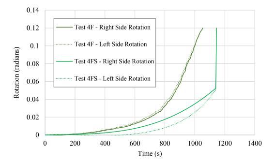
Figure 5.12 Time-rotation relationships showing the effect of perpendicular STS strengthening on the rotational resistance of connections with six bolts and five-times bolt end distance.
