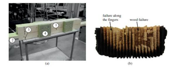
Figure 2.31 (a) Test specimen, finger joint (1), testing board (2), external lamellas (3) and insulating material (4); (b) Three-sided exposure of finger joint (Adapted from Klippel et al., 2013).
