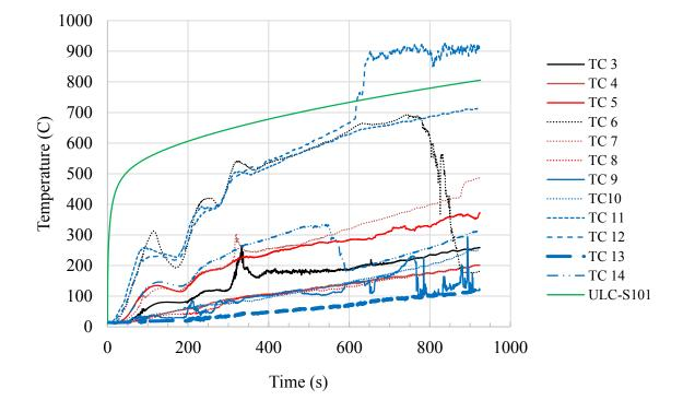
(c) Test 3F (four-bolt connection with five-times bolt diameter end distance).
