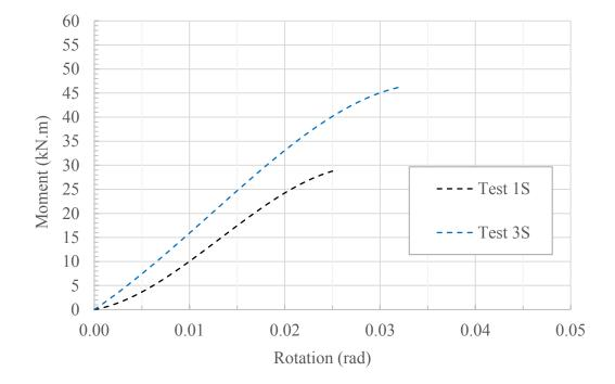
Figure 4.3 Moment-rotation relationships of test assemblies 1S and 3S using four bolts with four and five-times bolt dia. end distance, respectively.
