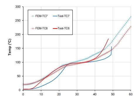
Figure 2.35 Comparing FEM and experimental temperatures of steel plate over time. (Adapted from Martin and Tingley, 2000).
