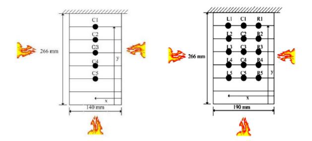
Figure 2.28 Test Group 6F (left) and 8F (right) (Adapted from Yang et al., 2009).
