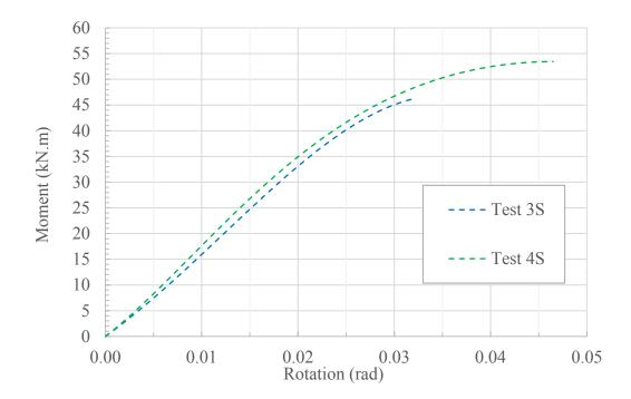
Figure 4.8 Moment-rotation relationships of test assemblies 3S and 4S using four and six bolts with five-times bolt dia. end distance, respectively (both STS-strengthened).
