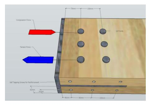
Figure 3.8 Steel connector with four-times bolt diameter end distance, six bolts and installation placement of STS strengthening.
