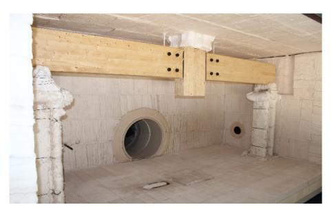
Figure 3.11 General beam-to-column test assembly inside the furnace with thermocouples and instrumentation installed.
