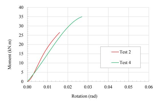
Figure 4.2 Moment-rotation relationships of test assemblies 2 and 4 using six bolts with four and five-times bolt dia. end distance, respectively.
