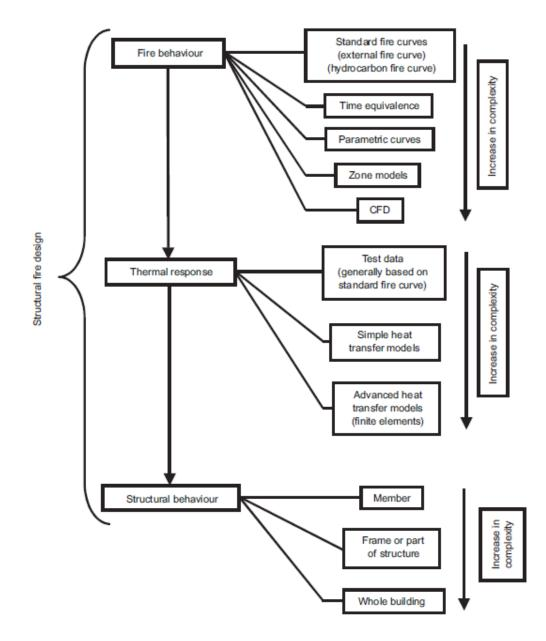
Figure 2.37 Increasing complexity of performance model with introduction of additional options (Adapted from Bailey, 2006).
