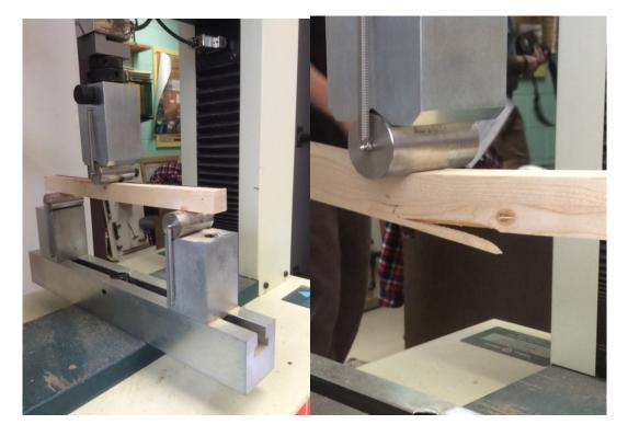
(a) Three-point flexural bending test.
