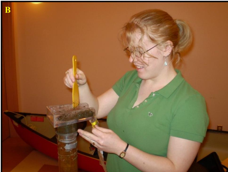
**Figure 5.6** Sampling the short core, WTFSH08-02, to be sub-sampled later for pollen and phytoliths processing in the lab.
