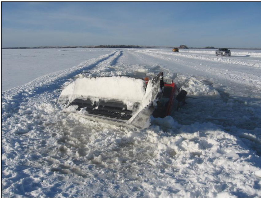
Figure 3.0 Snowplough going through the ice. Photo taken January 2011 on the winter road between Muskrat Dam and Sachigo Lake. Source withheld; printed with permission.
