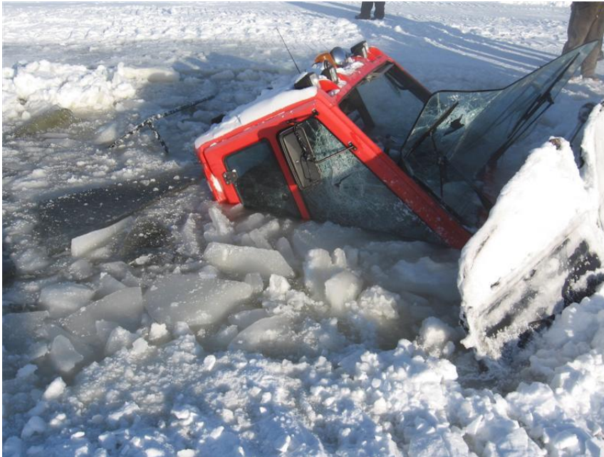
Figure 6. Snowplough fallen through the ice. Photo taken January 2011 between Sachigo Lake and Muskrat Dam, Ontario (west region). The reduction in the strength of the ice for winter road transportation is attributed to the absence and/or decreased depth of “blue-ice” formation. Source withheld; printed with permission.
