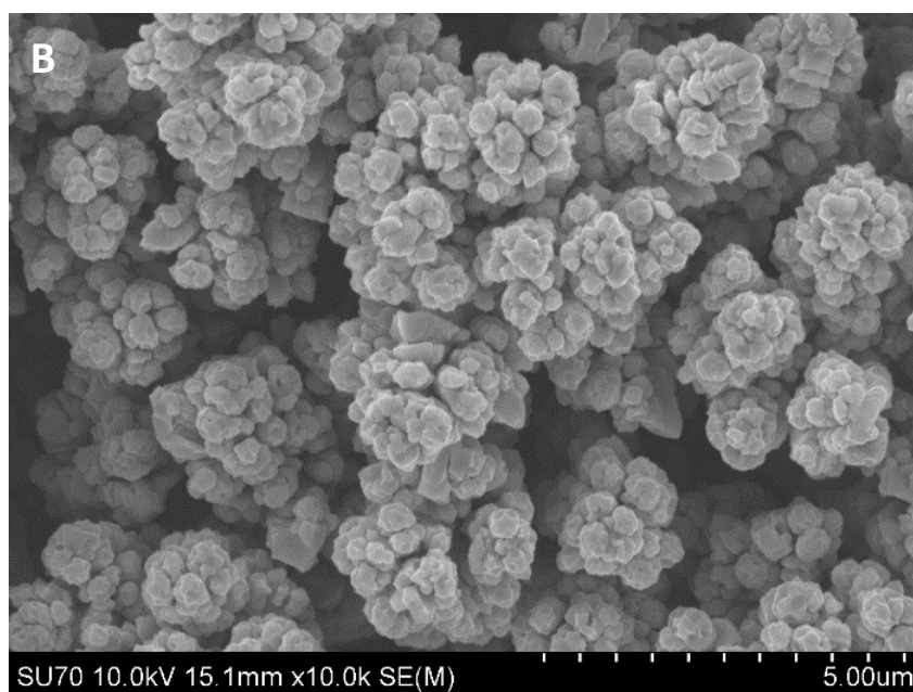
Figure 7.1 (A) & (B) SEM images of the 3D porous Ni grown on a Ni substrate via hydrogen bubble template electrochemical deposition at 3.0 \text{ A cm}^{-2} and 150 s.
