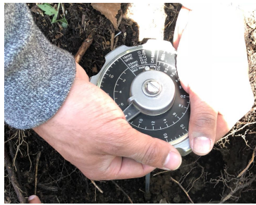
Figure 4.6: Vane shear test on the Nipigon slope
