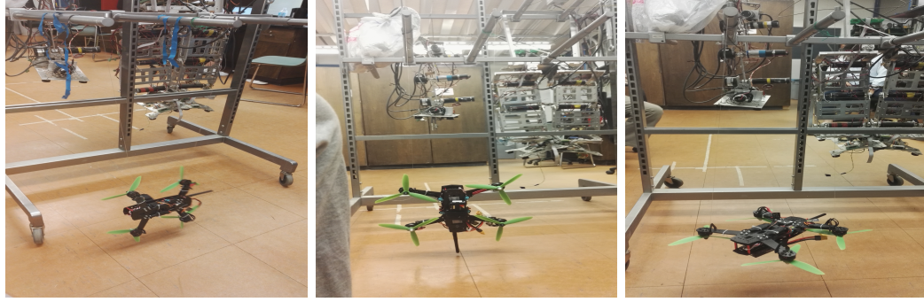
Figure 2.1: Measuring the Moment of Inertia
