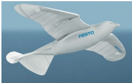
Figure 1.7: Festo's "SmartBird" Flapping Wing UAV
