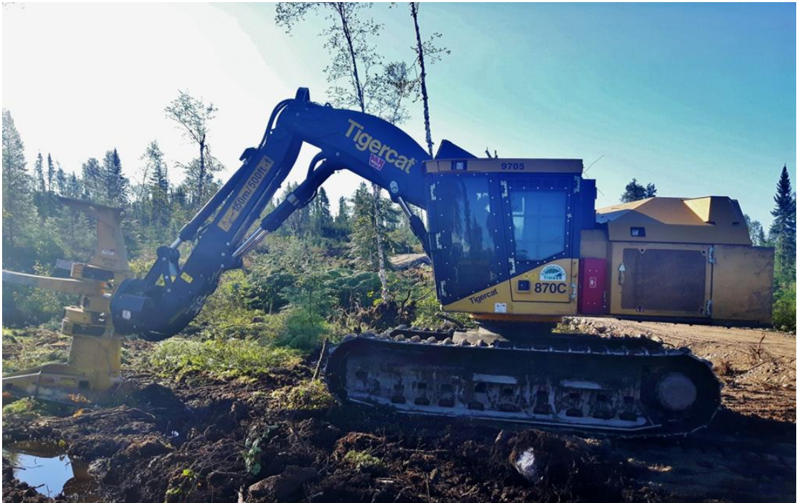
Figure 2. Tigercat 870C feller-buncher monitored in study.
