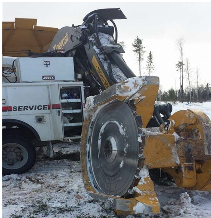
Figure 4. Felling head and circular saw on Tigercat 870C feller-buncher.
