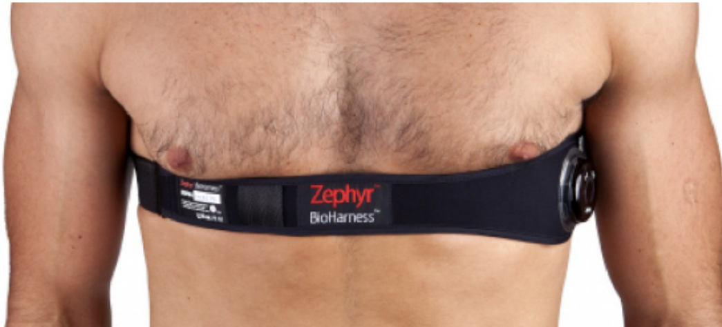
Figure 5. Positioning for Zephyr BioHarness Monitor. Diagram demonstrating the position to apply the Bioharness to properly monitor cardiovascular responses.
