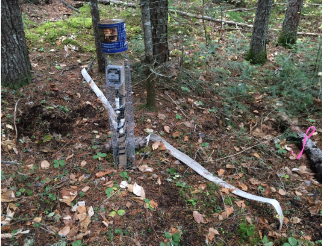
Figure 3. Hobo H21-002 Microclimate Data Logger site set up.
