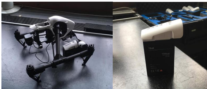
Figure 5. DJI Inspire drone and removeable rechargeable battery.
