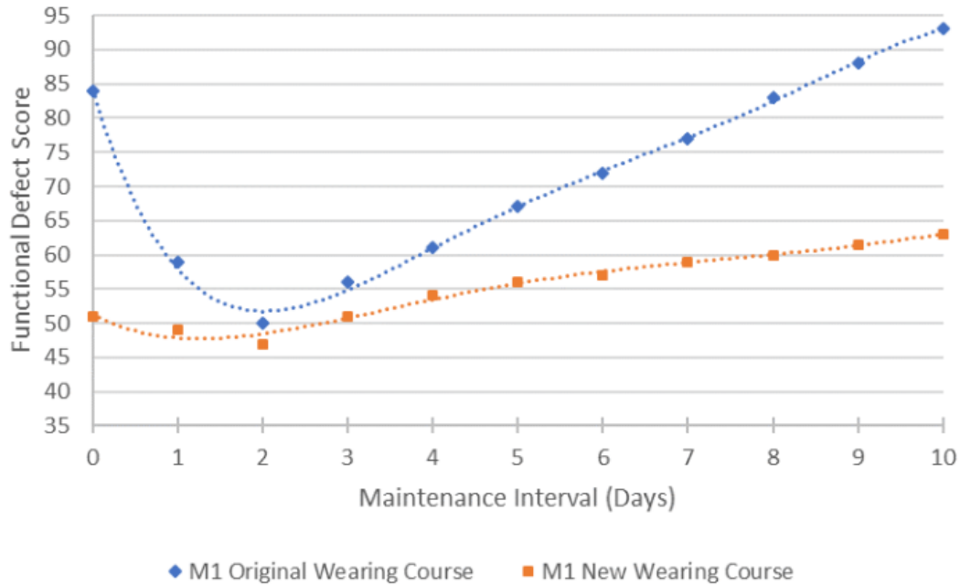
Figure 4. Predicted variation of functionality for original and optimised wearing course materials (Thompson and Visser, 2000)
