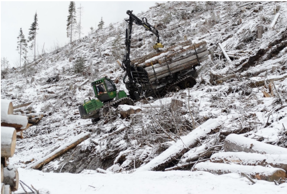
Figure 5. John Deere 1910E forwarder traveling loaded down a slope.
