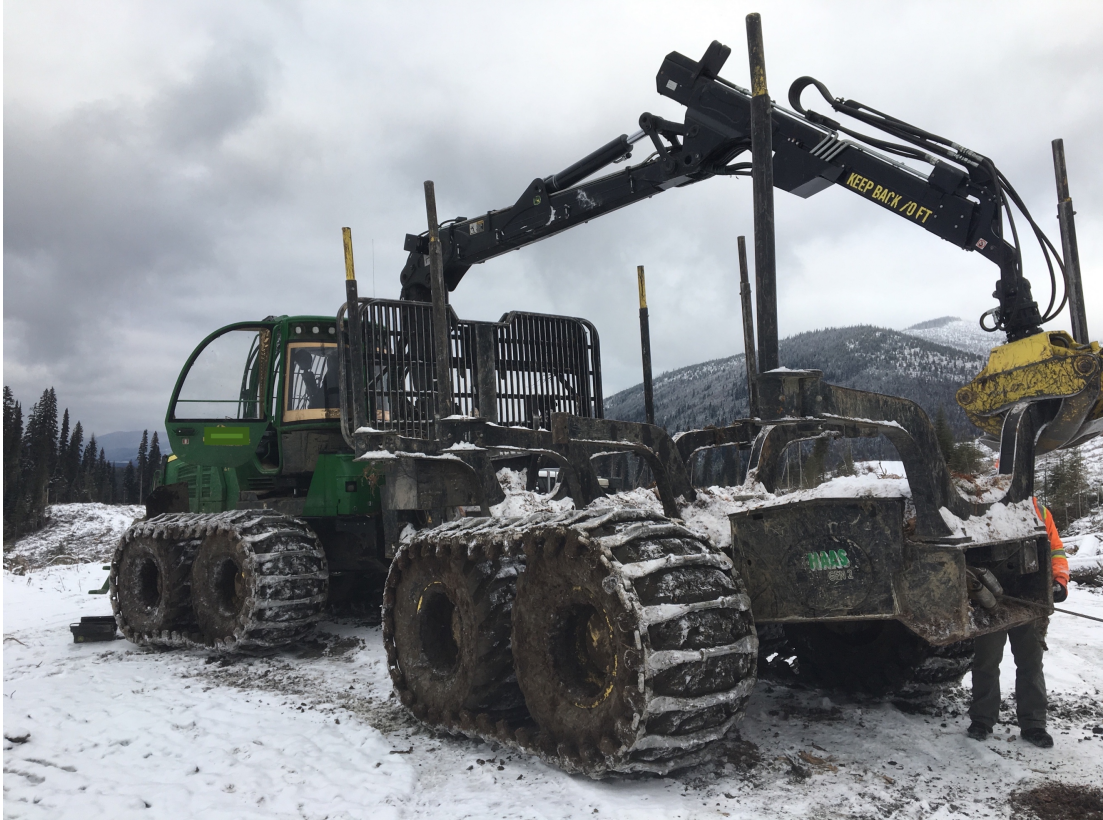
Figure 1. John Deere 1910E forwarder with Haas traction winch.
