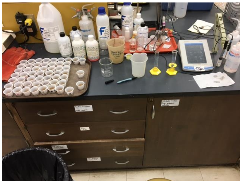
Figure 7. Materials used to measure soil pH: 10g soil samples (far left), graduated cylinders (centre right), and the pH machine (far right).
