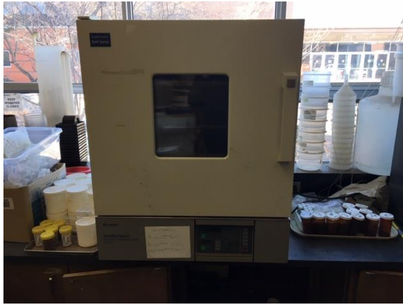
Figure 6. The drying oven that dried soil samples used to measure bulk density.
