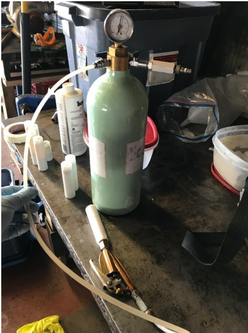
Figure 13. The full TreeAzin injection system setup with pressurized cylinder and cannisters.
