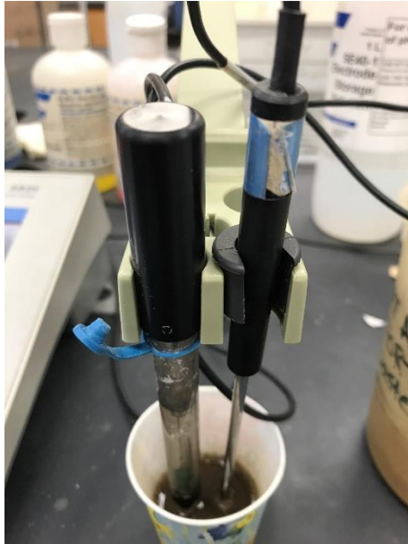
Figure 6: Temperature adjustment and an Orion 9165BNWP Sureflow Combination pH electrode used to measure samples pH.
